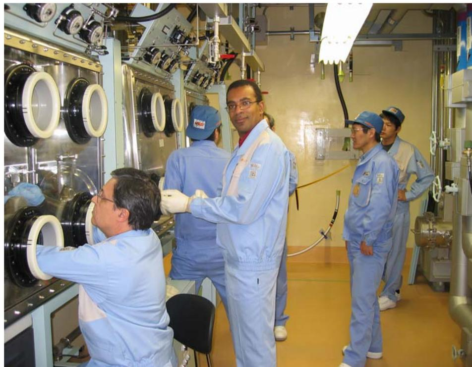
Sample loading for mass spectrometry measurements at Rokkasho reprocessing plant.
