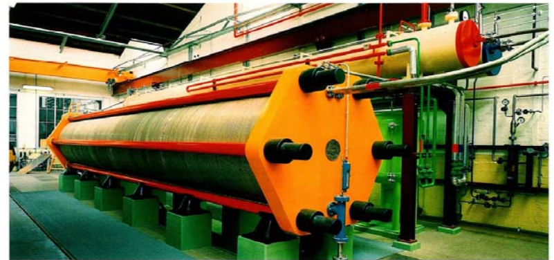
Pressure electrolyzer (Lurgi System) for hydrogen production, capacity 760 \text{ Nm}^3/\text{h H}_2
