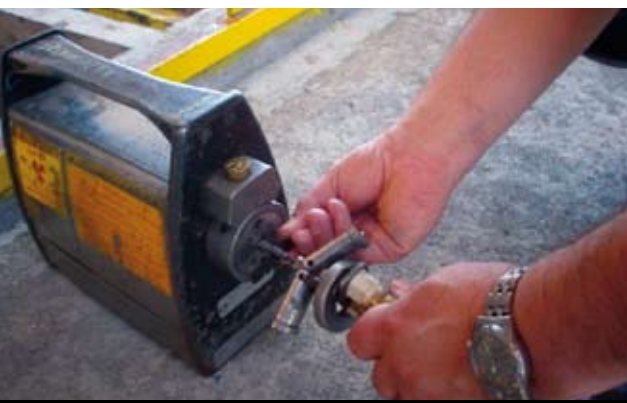
Typical iridium-192 shielding device.
