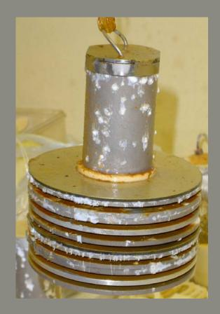
A test rack with coupons, before and after exposure for a year to a spent fuel basin in Serbia.
