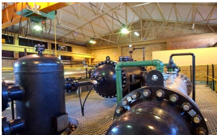
From Left to right: HPTU Main test vessel, Blower vessel, Water cooler
