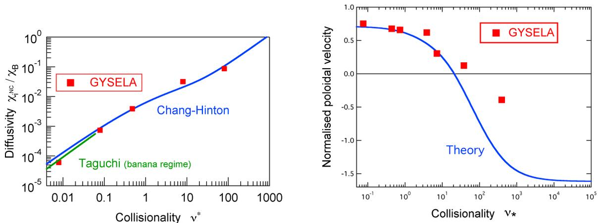
Figure 3: (left) Neoclassical normalised poloidal velocity and (right) neoclassical diffusivity as function of  $\nu_*$ , as computed with GYSELA. The straight lines refer to the neoclassical theoretical predictions.
