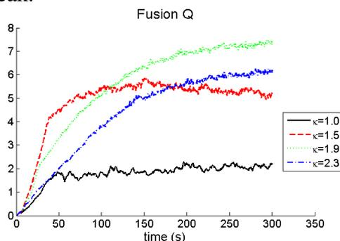
Figure 2: Elongation dependence of fusion  $Q$ , shown as time evolution profiles. MMM95 model is used.
