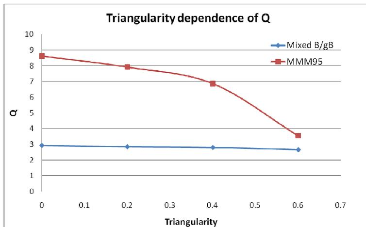
Fig. 5: Triangularity dependence of fusion Q at the end of the cycle, computed by the Multi-Mode Model and the Mixed Bohm/gyro-Bohm.
