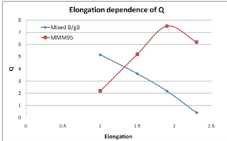
Fig. 4: Elongation dependence of fusion Q at the end of the cycle, computed by the Multi-Mode Model and the Mixed Bohm/gyro-Bohm.
