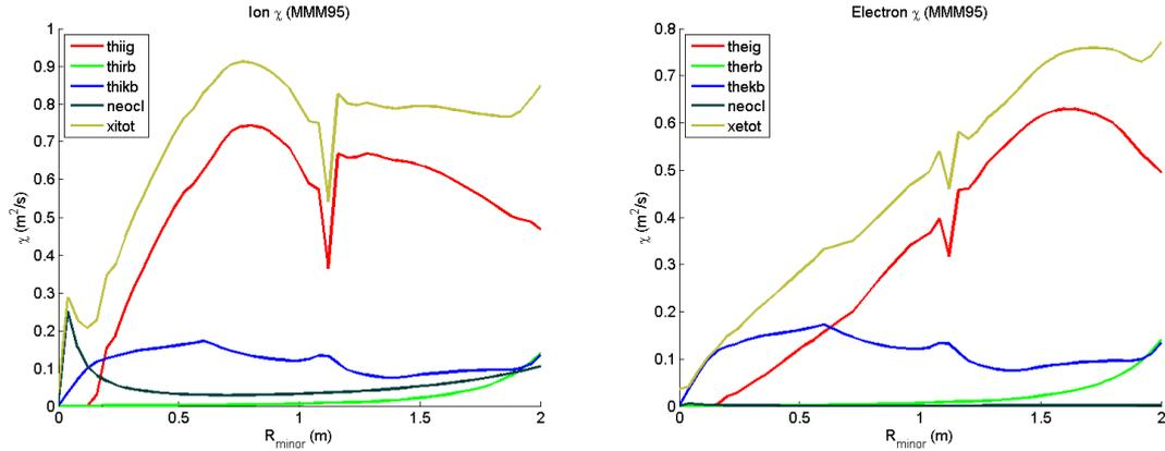
Figure 6: Ion thermal diffusivity and electron diffusivity (in m<sup>2</sup>/s) plotted as functions of minor radius at 300 sec. The transport is calculated using MMM95 model. The ITG and TEM contributions for the ions are labeled “thiig,” kinetic ballooning “thikb”, neoclassical “neocl,” total “xitot.” For the electron the “i” is replaced with “e.”
