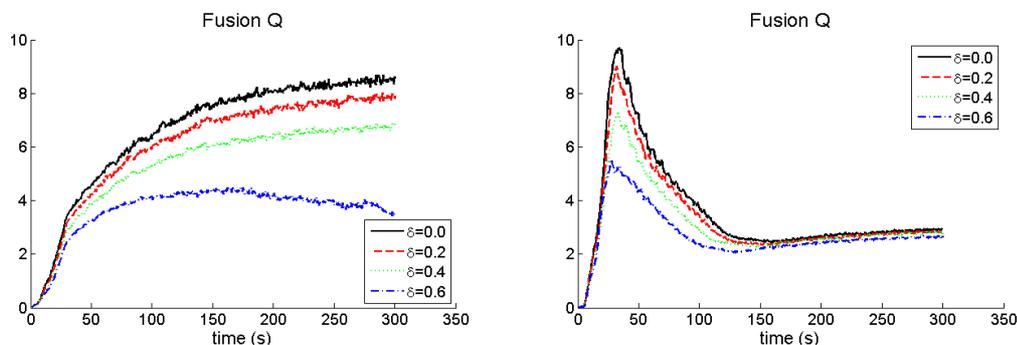
Figure 3: Triangularity dependence of fusion  $Q$ , shown as time evolution profiles. MMM95 model is used in the left panel. Mixed B/gB model results are shown on the right panel.
