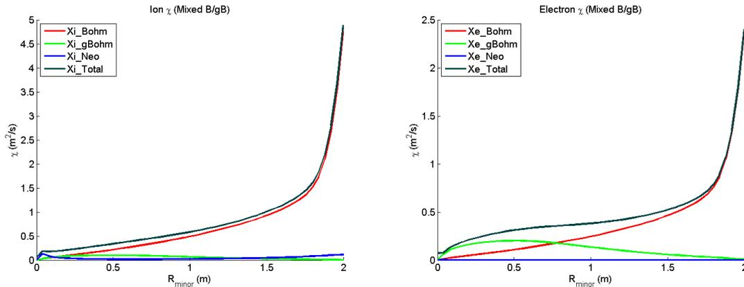
Figure 7: Ion thermal diffusivity and electron diffusivity (in m<sup>2</sup>/s) plotted as functions of minor radius at 300 sec. The transport is calculated using Mixed B/gB model. For the ion, the Bohm contributions are labeled “Xi\_Bohm,” gyro-Bohm “Xi\_gBohm”, neoclassical “Xi\_Neo,” total “Xi\_Total.” For the electron the “i” is replaced with “e.”
