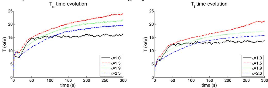
Figure 1: Time evolution of the electron (left) and ion (right) temperatures at the plasma core. MMM95 model is used.
