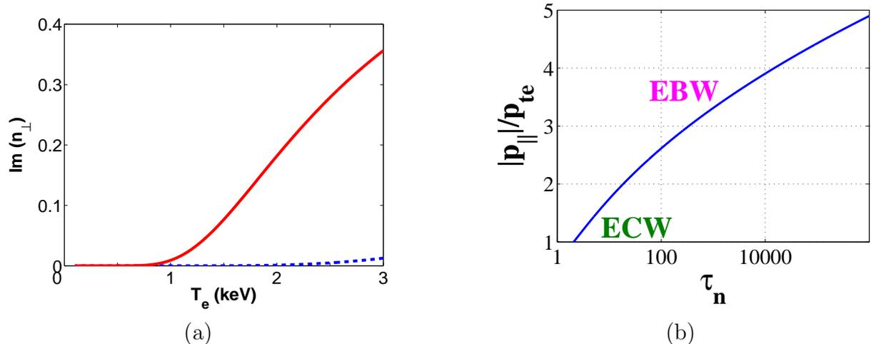
Figure 2: (a)  $Im(n_{\perp})$  versus electron temperature for NSTX-type plasmas with  $\omega/\omega_{ce} = 1.9$ ,  $\omega_{pe}/\omega_{ce} = 6$ , and  $n_{\parallel} = 0.2$ ; (b) The parallel electron momentum normalized to the thermal momentum versus the optical depth for the electron cyclotron waves. ECW represents the X and O waves.
