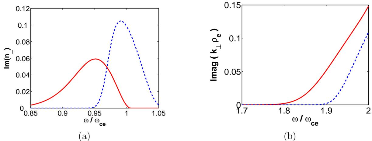
Figure 1: (a) Imaginary- $n_{\perp}$  for an O wave versus  $\omega/\omega_{ce}$  for ITER-type parameters with  $\omega/2\pi = 170$  GHz, electron temperature  $T_e = 10$  keV,  $\omega_{pe}/\omega = 0.75$  ( $\omega_{pe}$  is the electron plasma frequency), and  $n_{\parallel} = 0.1$ ; (b) imaginary part of  $(k_{\perp}\rho_e)$  for an EBW versus  $\omega/\omega_{ce}$  for NSTX-type parameters with  $\omega_{pe}/\omega_{ce} = 6$ ,  $T_e = 3$  keV, and  $n_{\parallel} = 0.2$ .
