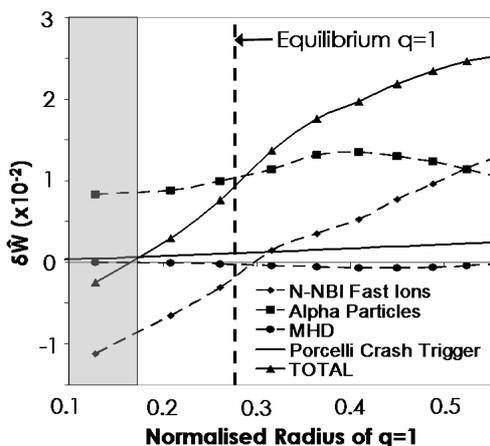
FIG. 4.  $\delta W$  due to energetic ions in ITER off-axis N-NBI heated plasmas as a function of  $r_1$ . When  $r_1$  is sufficiently core localised the off-axis N-NBI can destabilise the kink mode.
