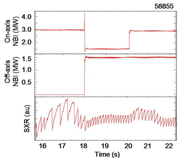
FIG. 2. Sawtooth destabilisation from the application of off-axis NBI in JET shot 58855.
