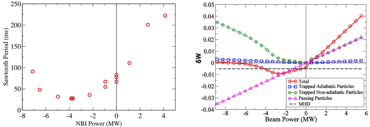
FIG. 1. The sawtooth period in JET NBI-heated plasmas compared to the stability of the  $n = 1$  internal kink mode.
