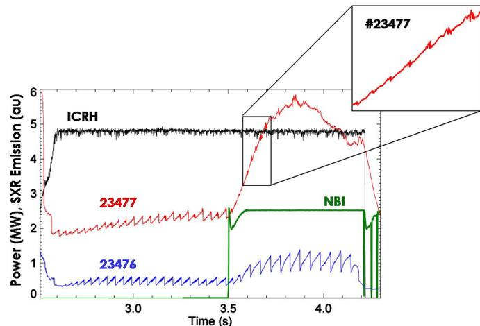
FIG. 3. ASDEX Upgrade shots 23476 and 23477 show a change in sawtooth behaviour when the NBI is injected near or well outside the  $q = 1$  surface respectively.
