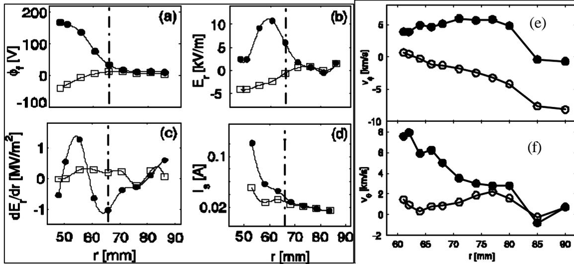
*Fig.2. Radial profiles of floating potential (a), radial electric field (b), the  $E_r$  shear, (c) ion saturation current (d), toroidal,  $v_\phi$ , (e) and poloidal velocity,  $v_\theta$  (f), averaged over 4 ms before (open symbols) and during (filled symbols) biasing. The vertical line marks the position of the LCFS.*
