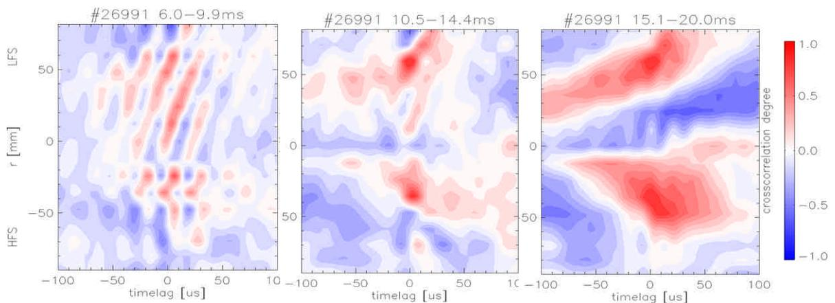
**Fig.3.** Cross-correlation between horizontal chord at 40 mm against all bottom chords prior to biasing (left figure), during biasing with biasing voltage +150V (middle figure) and after biasing (right figure).
