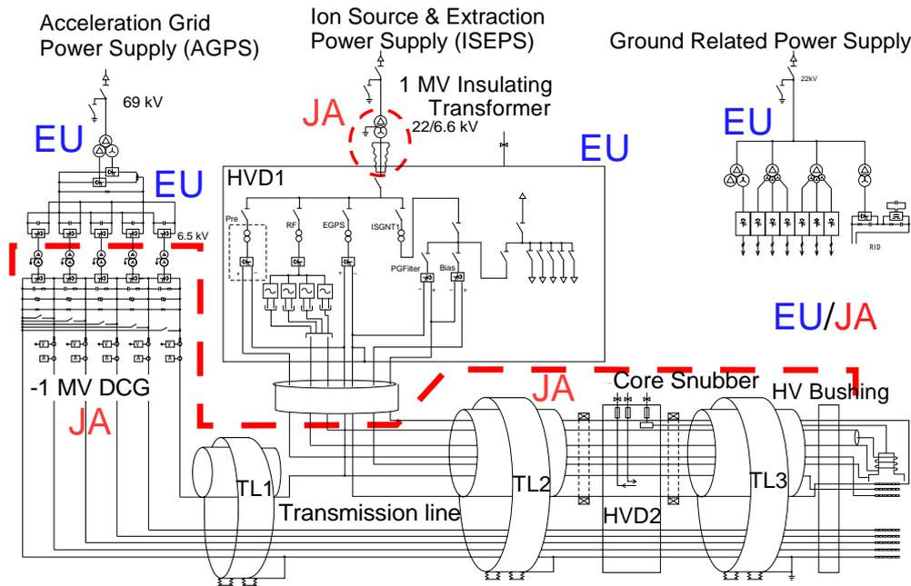
FIG. 1. ITER NBI Power supply system.
