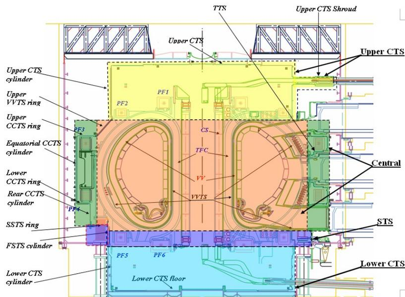
FIG. 1. Configuration of ITER thermal shield.
