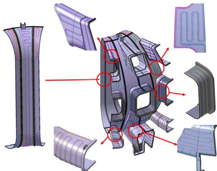
FIG. 3. Cooling line layout for ITER vacuum vessel thermal Shield.
