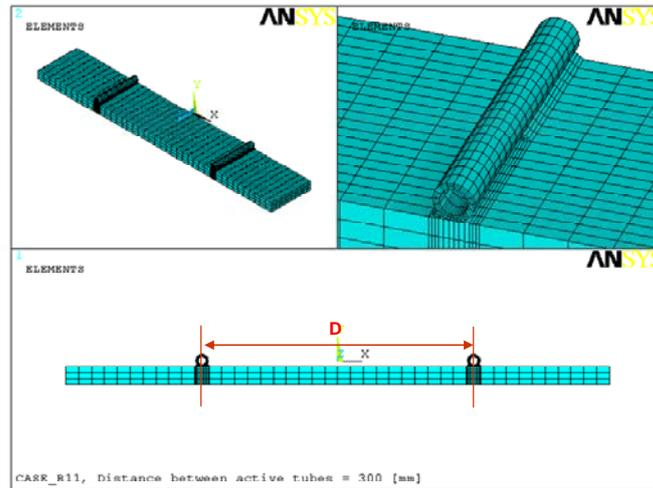
FIG. 6. Simplified FE model for thermal analysis.
