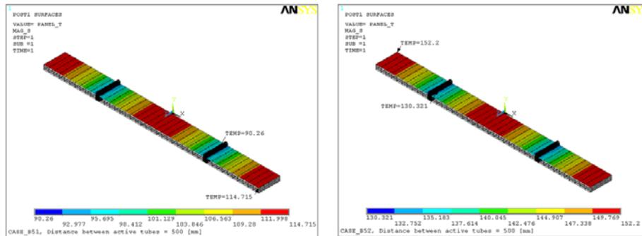
FIG. 7. Temperature distribution as the results of 3D simple model analysis .
