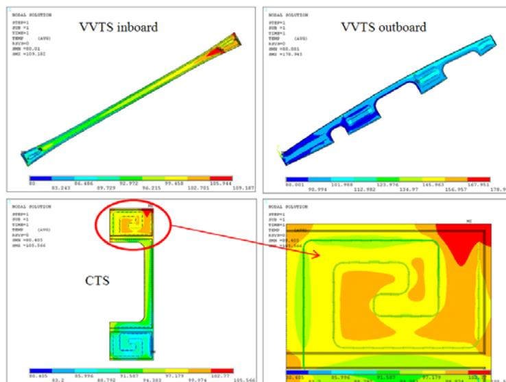
FIG. 8. Temperature distribution as the results of 3D full model analysis.
