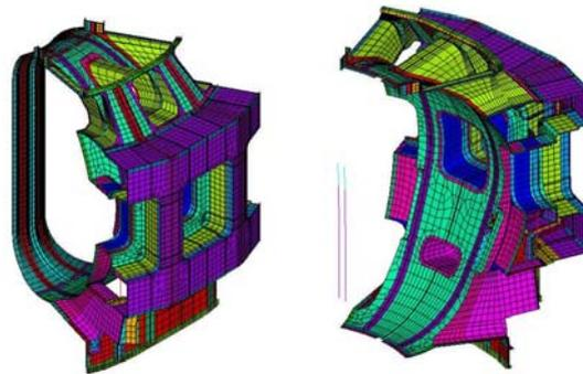
FIG. 4. FE model of equatorial thermal shield.
