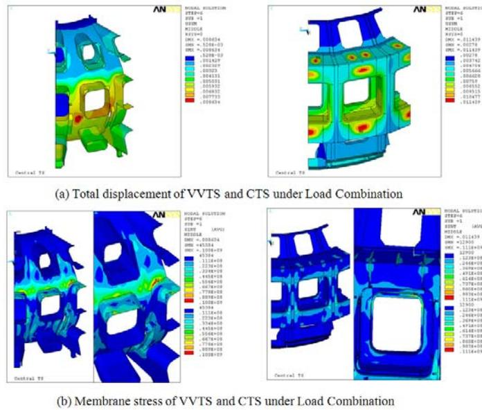
FIG. 5. Results of structural analysis for equatorial thermal shield under load combination.
