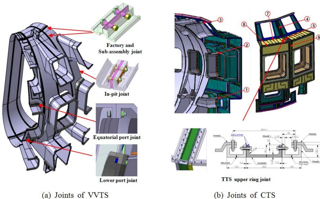
FIG. 2. Design of joints for ITER thermal shield.
