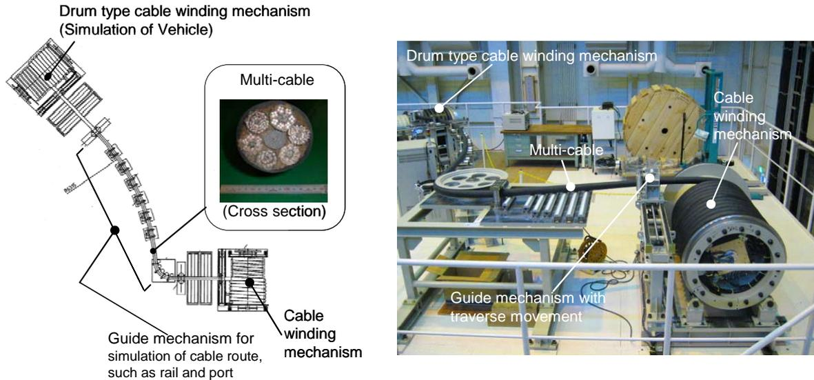
Fig. 9 Test facility of cable handling
