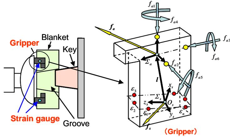
Fig.3 Forces acted on gripper during key insertion
