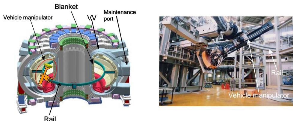
*Fig. 1 In-vessel Transporter for ITER*
