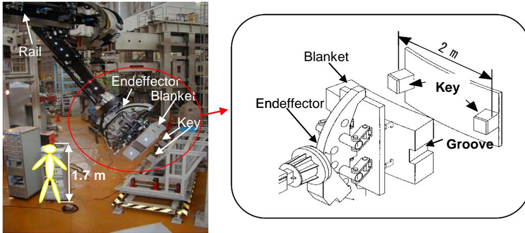
Fig.2 Installation of blanket module
