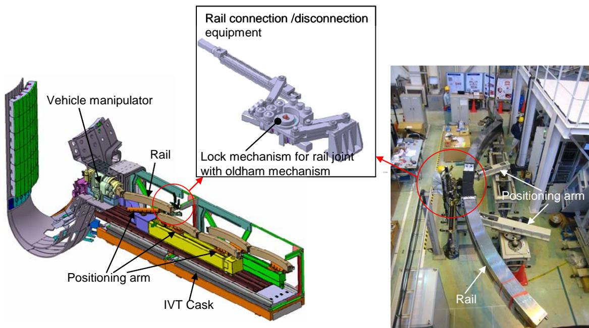
*Fig. 8 Test facility for rail connection and disconnection*
