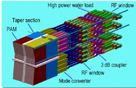
Figure 7: ITER 5GHz PAM Launcher concept [19].
