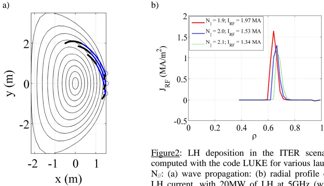
Figure 2: LH deposition in the ITER scenario 4 computed with the code LUKE for various launched  $N_{\parallel}$ : (a) wave propagation: (b) radial profile of the LH current, with 20MW of LH at 5GHz (with no electric field effect).
