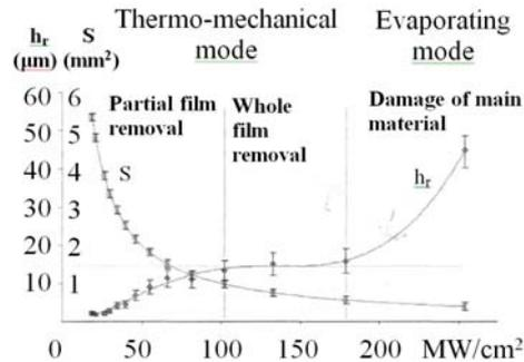
FIG.1. Experimental data for laser cleaning efficiency for removing of the corrosion layer from a steel plate. Profiles of the removed layer depth  $h_r$ , and the laser footprint area (equivalent to a laser power density, under the fixed energy parameters of laser pulse) demonstrate a gradual transition from thermo-mechanical to evaporating mode [14].
