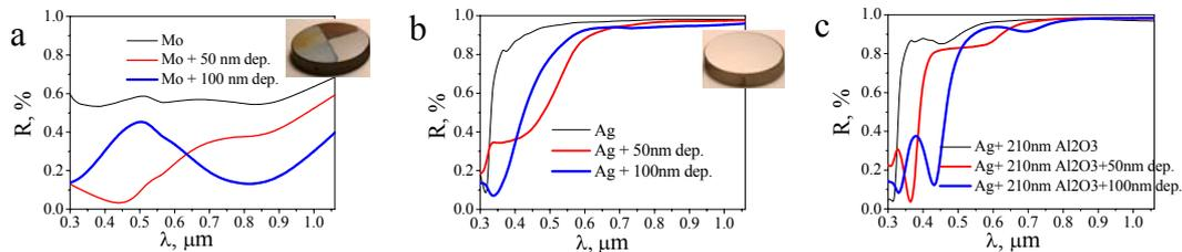
FIG.2. Reflection Spectra of Deposited Metal Mirrors (a) Mo , (b) Ag and (c) Ag protected by 210nm of  $\text{Al}_2\text{O}_3$  free of coating and with 50nm and 100nm thick deposits. All calculations were made for amorphous carbon deposited films and unpolarized emission reflected at  $45^\circ$  of incidence [21].
