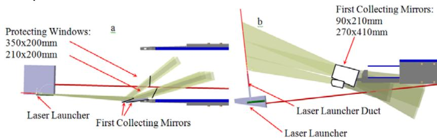
FIG.3. Layout drawing of the first optics TS in the divertor port (a) upper view, (b) side view.
