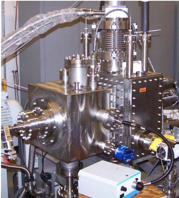
FIG. 3. Photo of pellet dropper device under test in ORNL pellet fueling laboratory.
