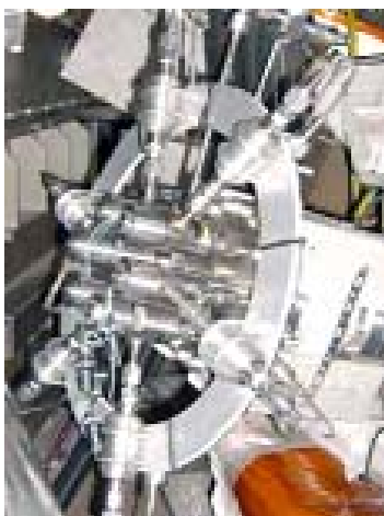
FIG. 6. Photo of the Medusa multi-valve gas jet system installed on the DIII-D tokamak.
