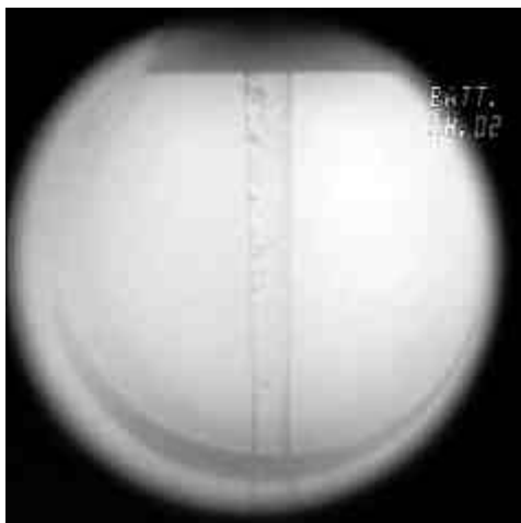
FIG. 2. Solid deuterium rectangular ribbon with a width of 3mm being extruded at a rate of 0.2 \text{ cm}^3/\text{s} from the prototype twin-screw extruder at a temperature of 16K.
