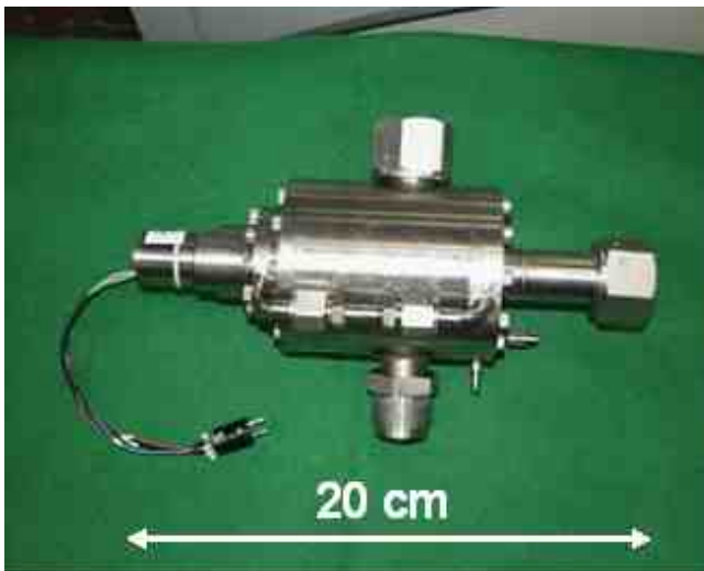
FIG. 5. High flow rate gas valve used for disruption mitigation testing. The valve orifice size is 22mm and has a maximum flow rate of 1 \times 10^7 mbar-L/s.
