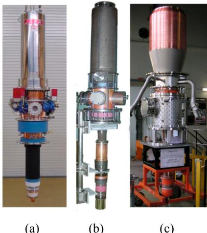
Fig.3 Picture of 170GHz gyrotrons. (a) Japan, (b) Russia, (c) Europe (coaxial gyrotron).
