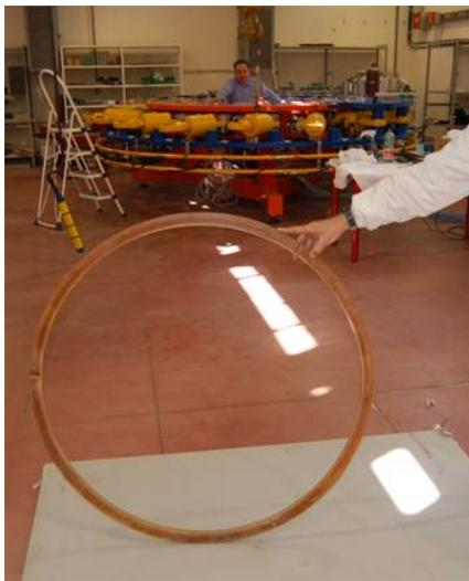
Fig. 9 Subsize pre-compression ring
