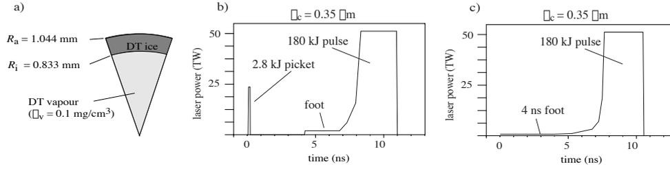
FIG. 1.: Reference capsule and laser pulses.
