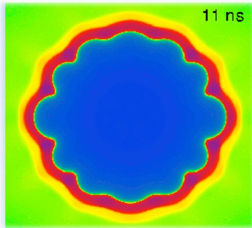
FIG. 3.: Multimode,  $90^\circ$ , CHIC simulation of the Hiper reference design. View of density contours just before time of maximum areal density ( $\approx 11.17$  ns).
