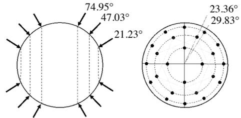
FIG. 2.: The 48 beams HiPER illumination scheme.
