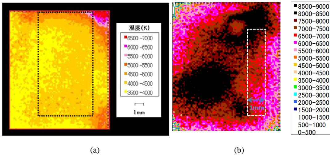
Fig. 1 Temperature distribution of discharge plasma. Front view (a), and side view (b)
