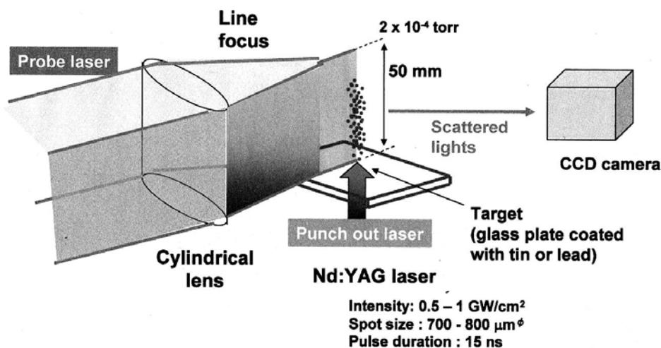
Fig. 5 Experimental setup to simulate ablation by particles that have Bragg peaks.
