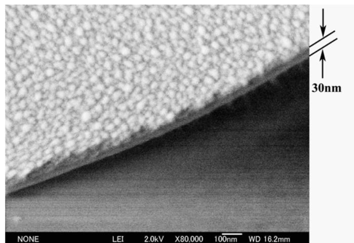
Fig. 2 Surface and cross section of deposited materials on a glass plate. There is continuous membrane under micro particles.
