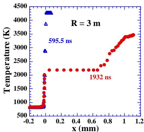
Fig. 7 temperature of ablated Pb in KOYO-F chamber
