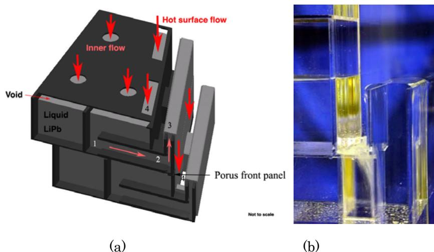
Fig. 9 Cascade scheme of KOYO-F (a) and mock-up experiment with water (b).
