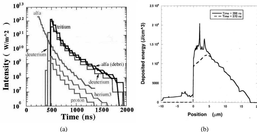
Fig. 4 Thermal loads by particles on the first wall of KOYO-F(a) and the energy deposition in Pb (b)
