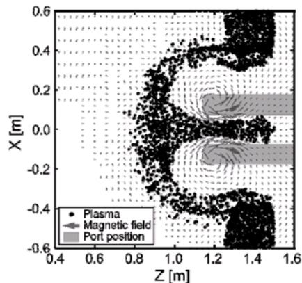
Fig. 8 Motion of alpha particles in a magnetic field for a port protection.
