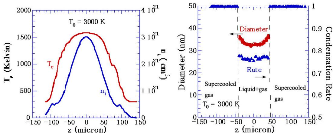
Fig. 3 Simulation on expansion of plasma from a 10  $\mu\text{m}$  thick, 3000K, free standing Pb membrane. The temperature and the density profile (a) and the diameter of aerosols (b) at 40 ns after the start of expansion..
