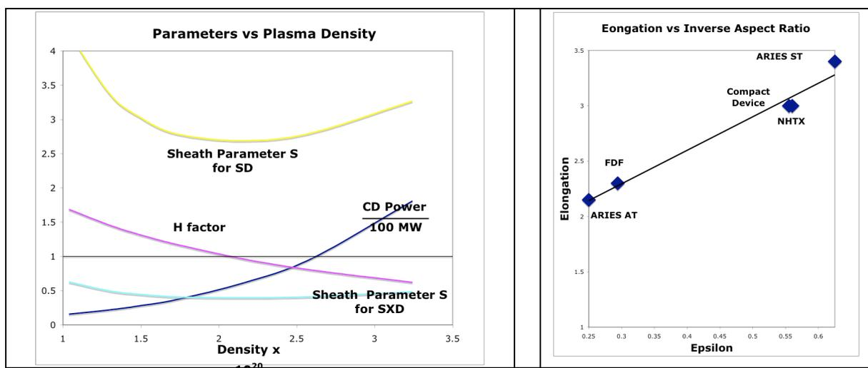
Fig. 4 Left: Parameters vs Density for the Compact 100MW fusion Device for  $\langle\beta\rangle_N=3$ . Right: Elongation vs Aspect Ratio for recently proposed devices
