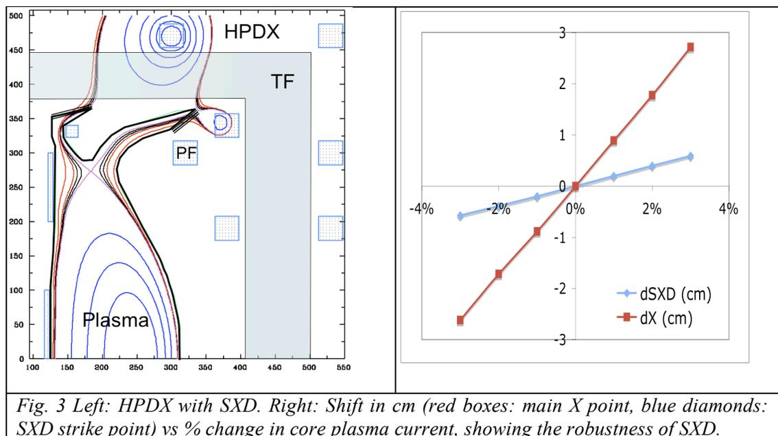
Fig. 3 Left: HPDX with SXD. Right: Shift in cm (red boxes: main X point, blue diamonds: SXD strike point) vs % change in core plasma current, showing the robustness of SXD.
