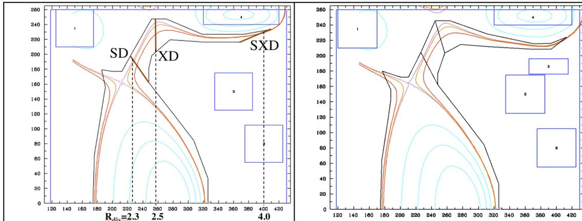
FIG 1. CORSICA SXD equilibria for FDF: Left: with 1 SXD coil (in top right corner of TF), Right: with 2 coils carrying same total current as the single coil.
