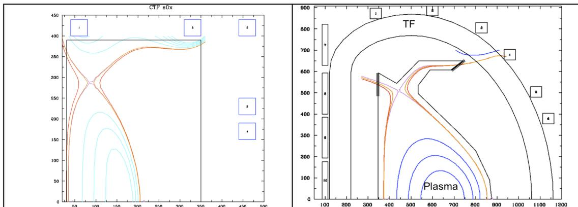
FIG 2. Left: SXD for low-A CTF, Right: SLIMCS reactor with SC PF coils outside TF.
