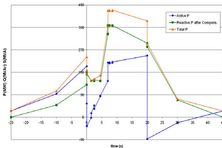
FIG. 9 -FAST Electric Power from the 400 kV grid
