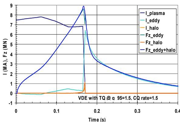
FIG. 6-VDE parameters and Fz EM force
