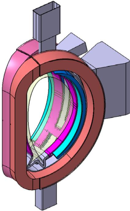
FIG. 2- Toroidal magnet module
