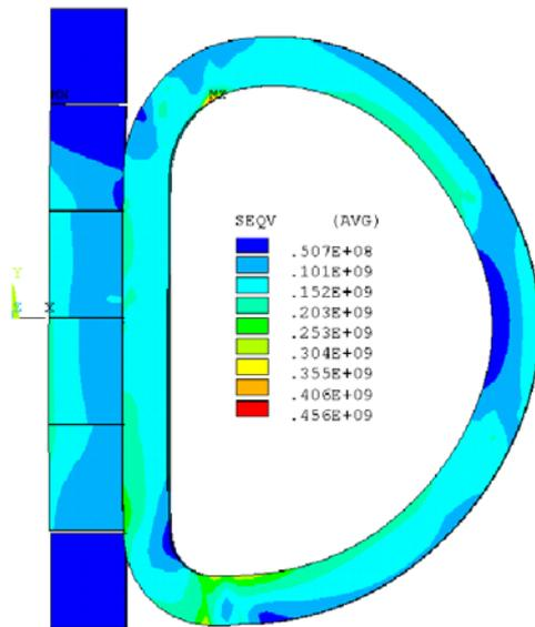
FIG. 4- VM stress (MPa) on copper
