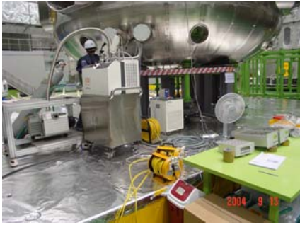
FIG. 3 VV 337.5° sector under leak test
