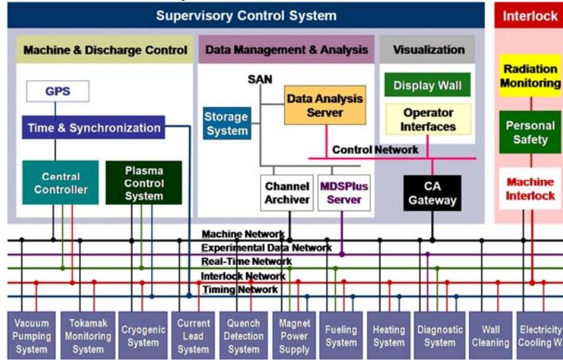
FIG. 1. Schematic of KSTAR Integrated Control System
