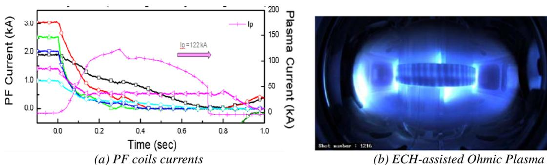
FIG. 8. Results of 1<sup>st</sup> plasma experiment of KSTAR
