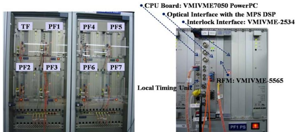
FIG. 3. Installation of VME-based MPS Local Control Systems
