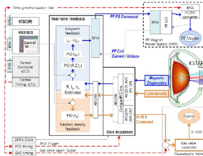
FIG. 4. Hardware Layout of PCS for the Day-I operation
