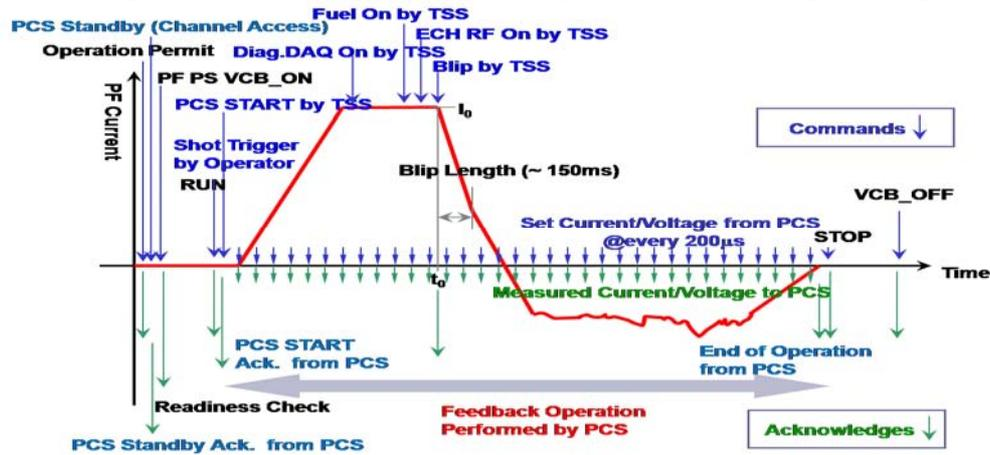
FIG. 7. Operation Sequence of Synchronized Real-time Feedback Operation
