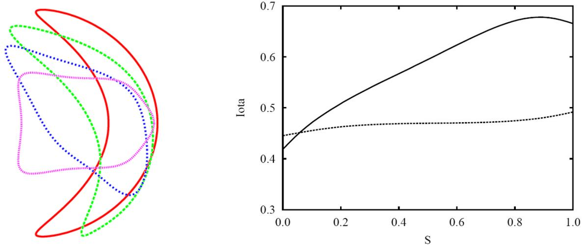
FIG. 2. A) Cross section of the LCMS at four toroidal sections and B) the rotational transform as a function of normalized toroidal flux  $s$  for the N3ARE configuration. The dashed line is the rotational transform from external coils (or transform at  $\beta = 0$ ) and the solid line is the total rotational transform (iota) including the bootstrap current contribution at  $\beta = 5\%$ .
