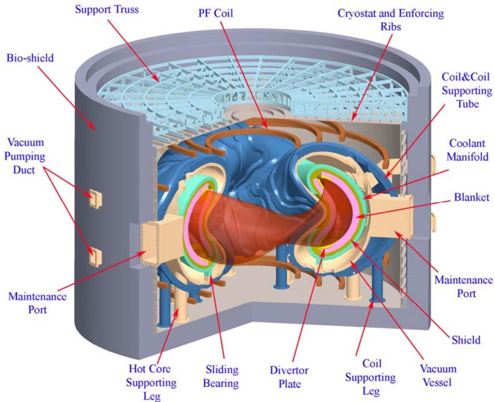
FIG. 1. The ARIES-CS fusion power core.
