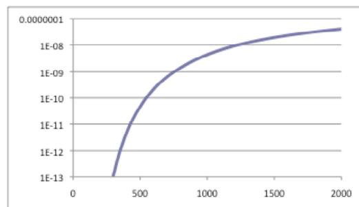
FIG 3. Diffusivity ( $m^2/sec$ ) of H in W vs. temperature (K).
