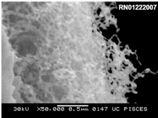
FIG. 1. Foaming of tungsten surface due to bombardment with helium.
