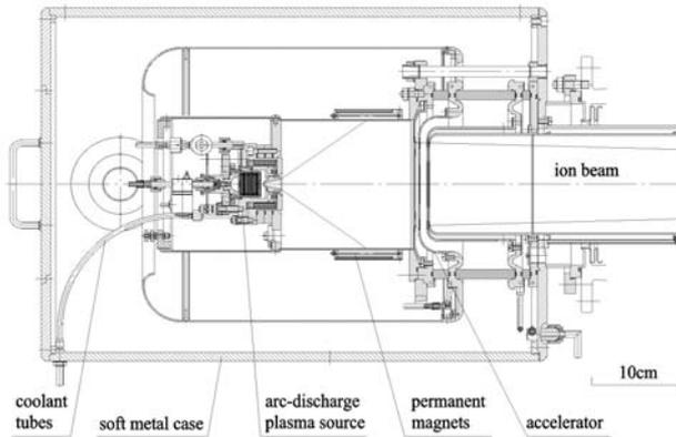
FIG. 1. Schematic view of ion source with an arc-discharge plasma box.
