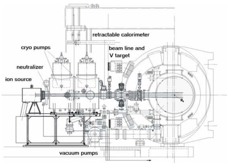
FIG. 2. Diagnostic neutral beam injector setup at TEXTOR.
