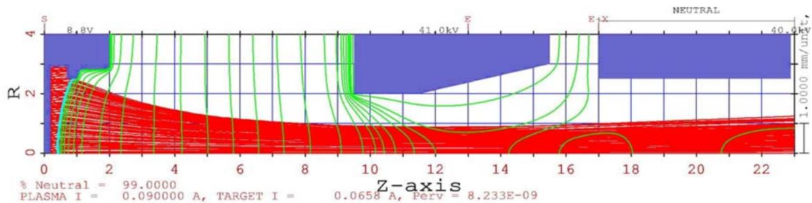
Fig.7 Plot of ion trajectories and equipotentials in elementary cell.
