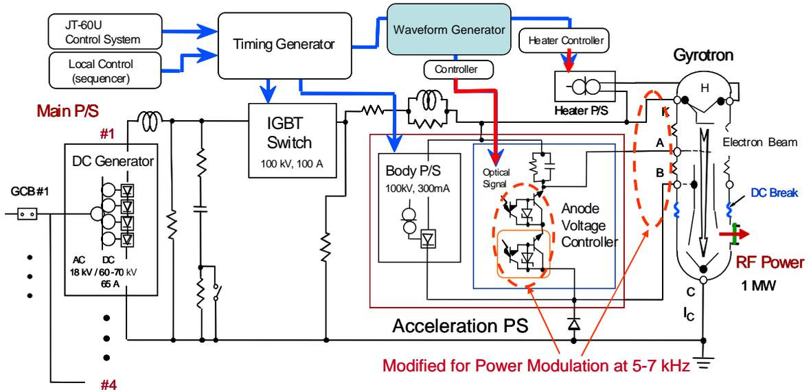
Fig. 9. Schematic diagram of power supply for long pulse gyrotron operation in JT-60U ECRF system.
