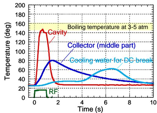
Fig. 4. Temperature of components in the gyrotron and cooling water on 1.5MW for 1s oscillation.
