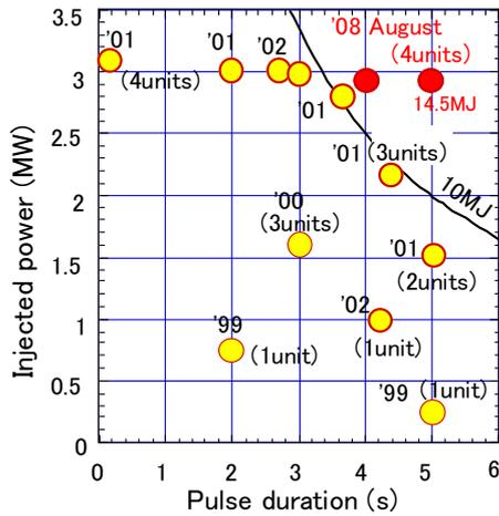
Fig. 1. Injected RF power and pulse duration of JT-60 ECRF system. Simultaneous operation of all 4 gyrotrons at 1MW for 5sec enabled 2.9 MW (14.5 MJ) injection with transmission efficiency of ~0.75.
