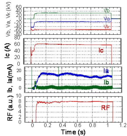
Fig. 2. Waveforms of high voltage applied to the gyrotron, current and RF signals on 1.5 MW for 1 s oscillation. The suffixes a, b, c, k stand for anode, body, collector and cathode respectively.
