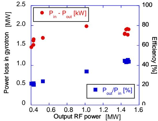
Fig.6. Gyrotron efficiency and power balance. Higher Gyrotron efficiency obtained with higher output power.
