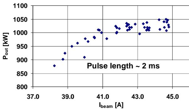
Fig. 4: Saturation of output power with increasing beam current measured with SN2.
