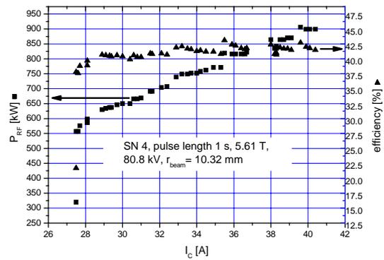
Fig. 2: Output power and efficiency of series gyrotron SN4 in dependence of beam current.
