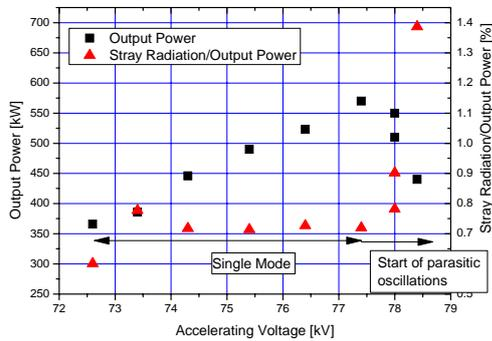
Fig. 6: Output power and relative stray radiation measured at the relief window versus accelerating voltage.
