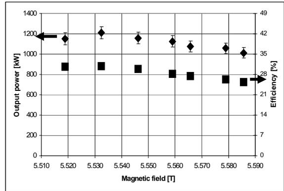
Fig. 5: Output power and efficiency SN2 achieved with 50 A beam current.
