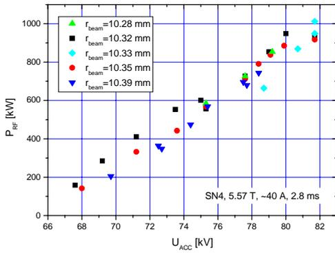
Fig. 1: Output power of SN4 gyrotron in short pulse versus accelerating voltage at different electron beam radii in the cavity.
