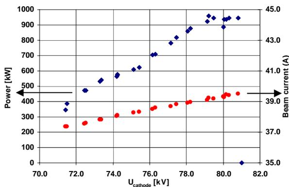
Fig. 3: Influence of accelerating voltage on output power and beam current in short pulse operation of SN2.
