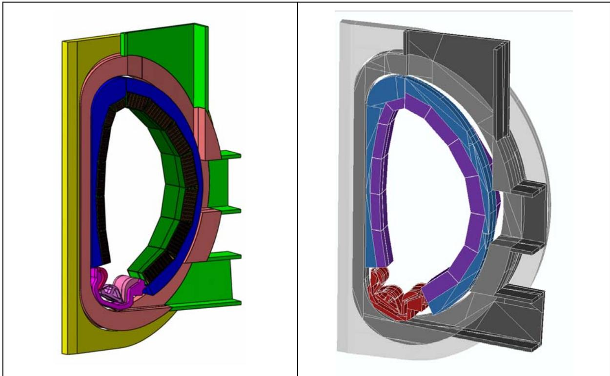
Fig. 2: DEMO torus sector model (11.25°) with integrated HCLL blanket modules for neutronics analyses: CAD model generated with CATIA V5 (left) and MCNP model converted and visualised by McCad (right)
