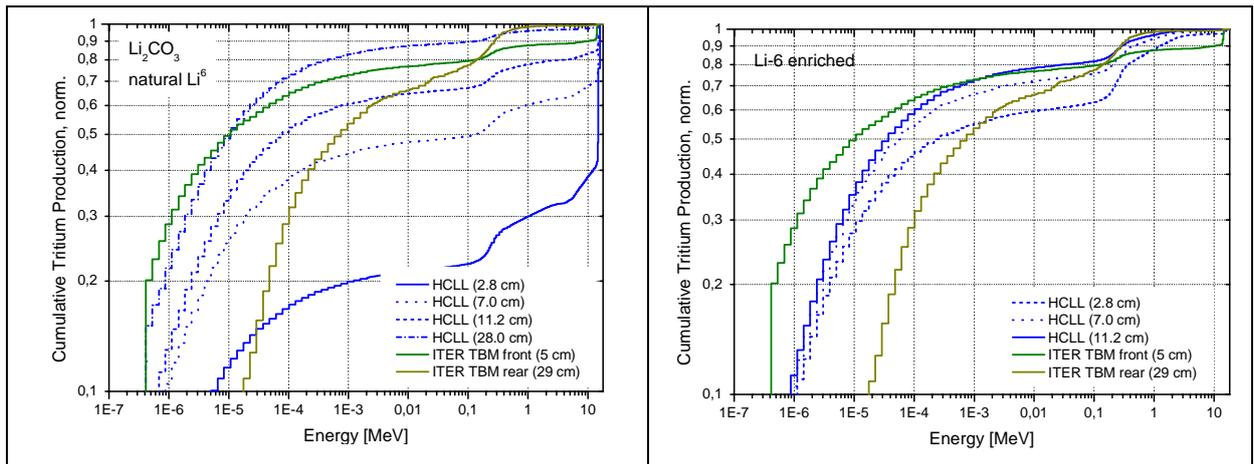
Fig. 4: Cumulative Tritium production rates in the HCLL mock-up compared to front and rear positions in the ITER TBM. The pellet detectors consist of  $\text{Li}_2\text{CO}_3$  with natural Lithium (left figure) and enriched Lithium (90 at%  $^6\text{Li}$ , right figure).
