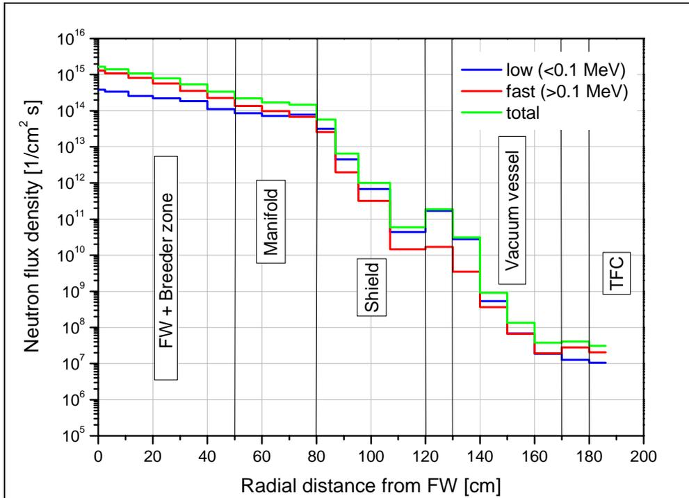
Fig. 1: Radial profiles of the neutron flux densities across the inboard mid-plane of the HCLL power reactor.
