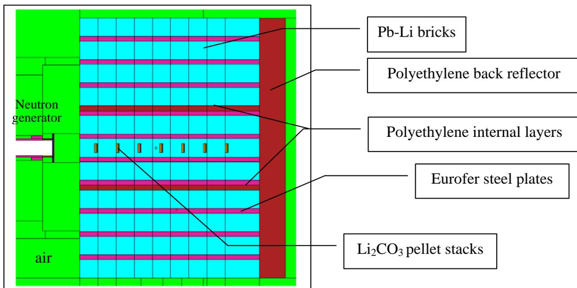
Fig. 3: HCLL TBM mock-up (MCNP model, vertical cut) showing the Pb-Li bricks, the Eurofer steel plates, the polyethylene layers and one row of  $\text{Li}_2\text{CO}_3$  pellet stacks.
