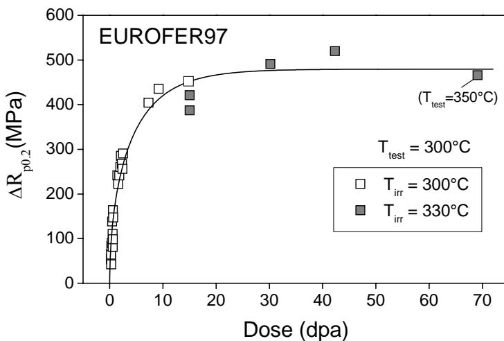
*FIG. 2.* Irradiation hardening vs. irradiation dose for  $T_{\text{irr}}=300$ -330 °C and  $T_{\text{test}}=300$  °C (exception: specimen from ARBOR 2 is tested at  $T_{\text{test}}=350$  °C) of EUROFER97. For comparative purposes the low dose data from [2,3] are also included. The line is a model description of the entire data set.
