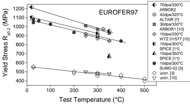
*FIG. 1.* Yield stress  $R_{p0.2}$  vs. test temperature for EUROFER97 in the unirradiated condition and after neutron irradiations in different European irradiation programmes (irradiation conditions and programmes are given in the figure legend). The lines are a guide for the eye.
