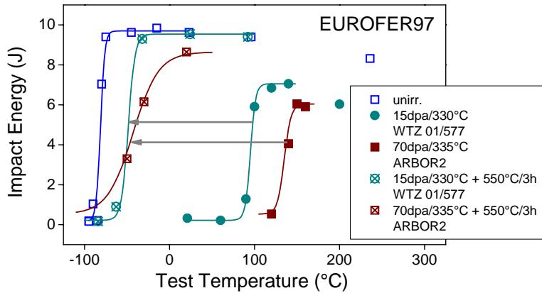
*FIG. 6. Impact energy vs. test temperature for EUROFER from the WTZ 01/577 and ARBOR 2 irradiations in the as irradiated condition and after post-irradiation annealing at 550 °C for 3 h. The results in the reference unirradiated condition are also included. The lines are fits to the ductile-to-brittle-transition regions as described in [5]. The arrows indicate recovery of the DBTT.*
