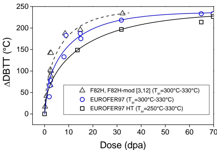
*FIG. 4. Irradiation shifts of the DBTT vs. irradiation dose for EUROFER97 and F82H steels. The irradiation temperatures are indicated in the figure legend. The solid lines are a model description of the data. The dashed line is a guide for the eye.*
