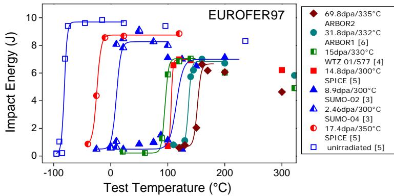
*FIG. 3. Impact energy vs. test temperature of EUROFER97 in unirradiated condition and after neutron irradiations in different European irradiation programmes (irradiation conditions and programmes are given in the figure legend). The specimens are machined from the as-delivered 25 mm plate. The lines are fits to the ductile-to-brittle-transition regions as described in [5].*
