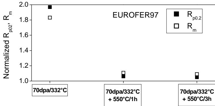
*FIG. 5. Yield Stress and ultimate tensile strength for irradiated EUROFER97 (ARBOR 2) normalized with respect to the corresponding unirradiated values in the as-irradiated condition and after post-irradiation annealing.*
