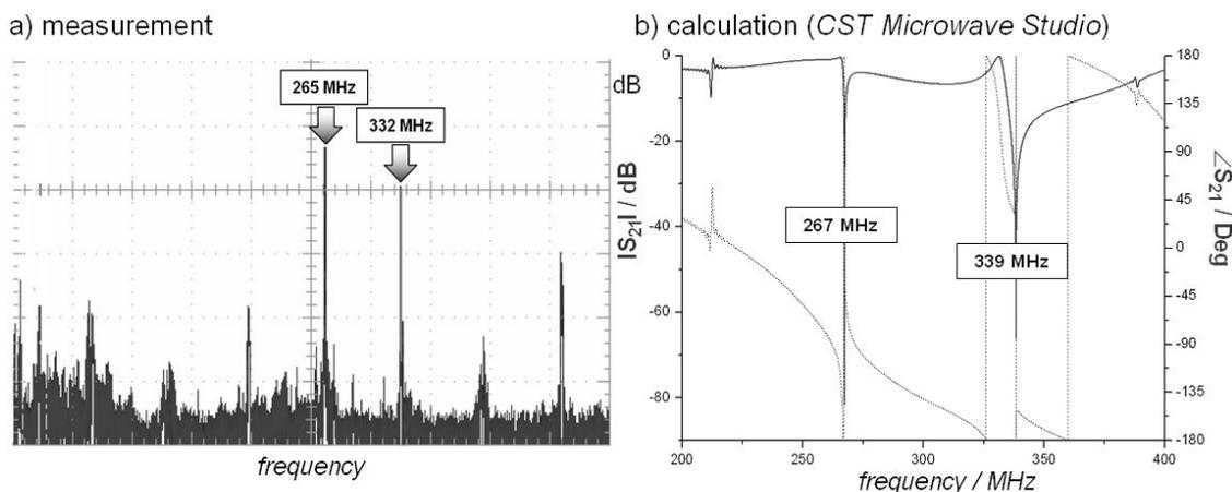
FIG. 1. Measured (LF) parasitic oscillations (a) and calculated with CST (b) frequency spectrum of the inner geometry of the pre-prototype gyrotron.
