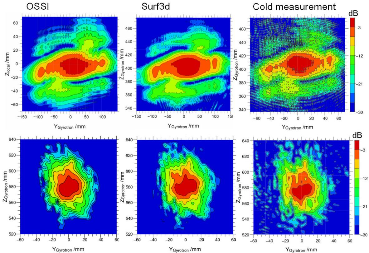
FIG. 6. Comparison of the measured fields patterns (right) with calculations: OSSI (left) and Surf3d (middle), at the 2<sup>nd</sup> mirror position (upper row) and on the gyrotron window (bottom row).
