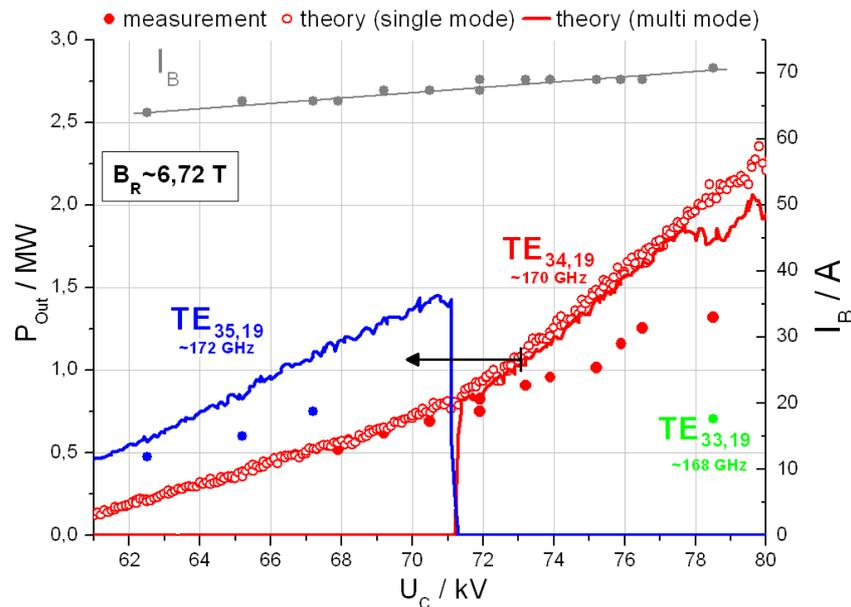
FIG. 3. RF output power vs. cathode voltage. The experimental values are compared with self consistent calculations (single and multi-mode).
