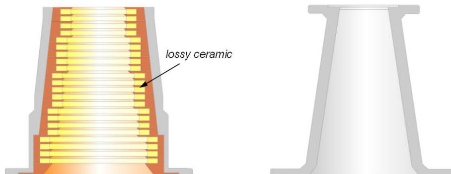
FIG. 4. Beam tunnels used in the experiments with pre-prototype gyrotron.
