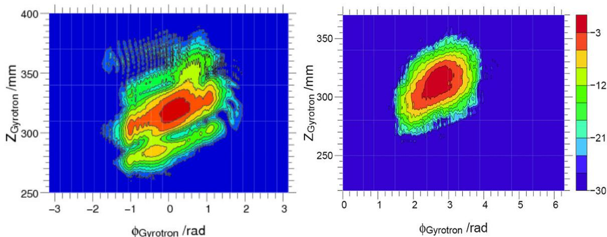
FIG. 8. Surf3d calculation of the radiated field of the: current launcher with 1<sup>st</sup>, 3<sup>rd</sup> perturbation orders at the inner wall (left) and improved launcher with arbitrary deformations (right).
