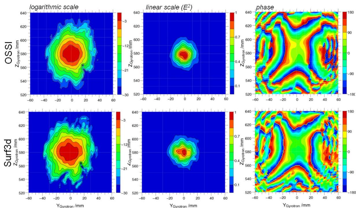
FIG. 7. Results of the optimization of the 3<sup>rd</sup> phase correcting mirror – field distribution at gyrotron window calculated with OSSI (upper row) and results of verification with Surf3d (bottom row).
