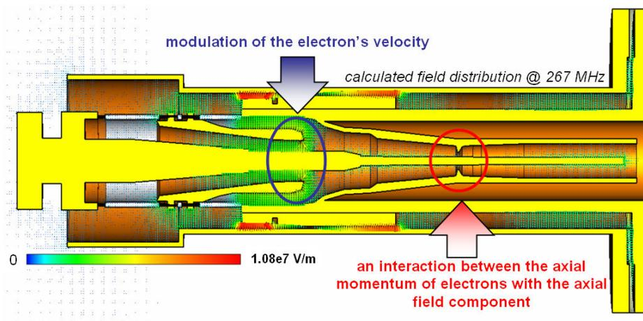
FIG. 2. Calculated field distributions at 267 MHz – regions responsible for the excitation of the parasitic oscillation are indicated.
