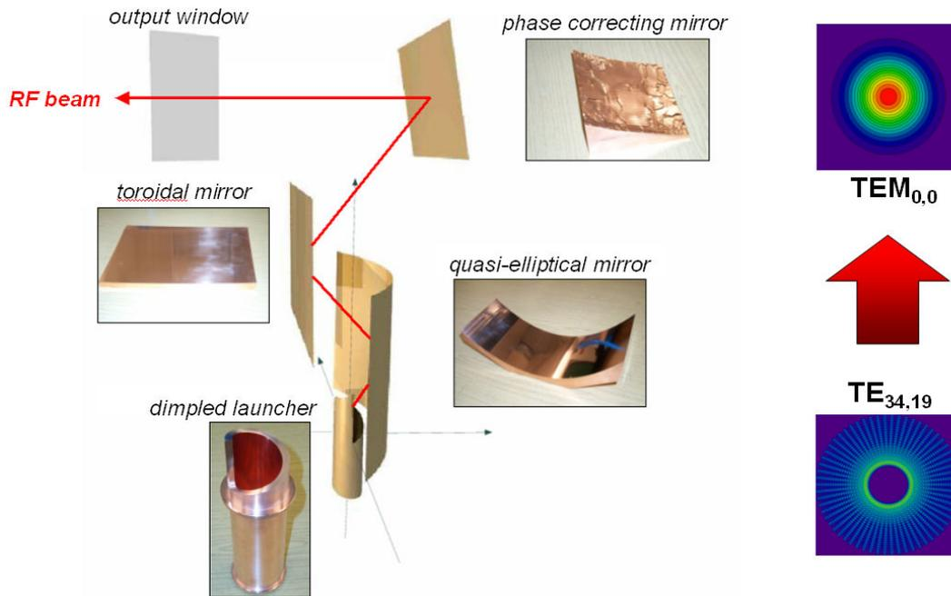
FIG. 5. Arrangement of the q.o. RF output system.
