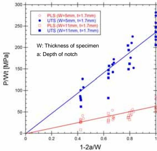
FIG.5. Example of failure evaluation of advanced SiC<sub>f</sub>/SiC composites by the double notch tensile test method.
