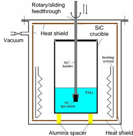
FIG. 6. Experimental apparatus proposed for the compatibility test between SiC materials and a Pb-17Li liquid metal.
