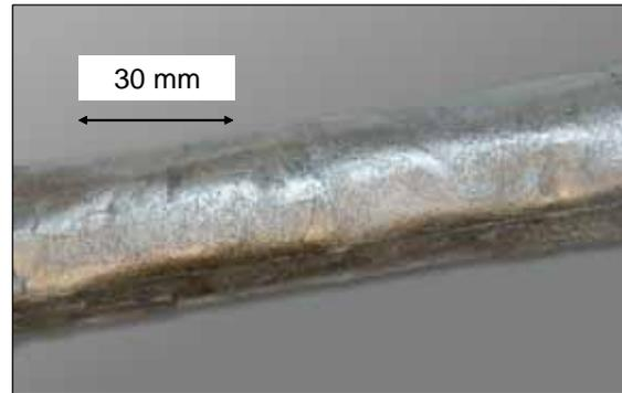
FIG.8 Picture of the large rods of Be-30.8 wt%Ti fabricated in FZK.
