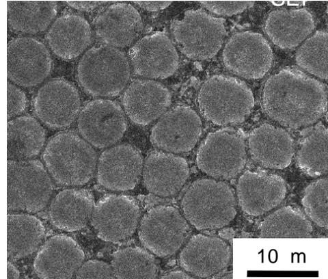
FIG. 4. Micro-structure of the unidirectional NITE-SiC<sub>f</sub>/SiC composite.
