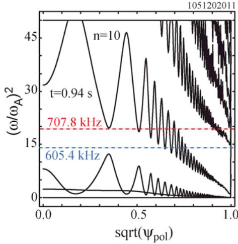
Fig. 4. NOVA calculated Alfvén continuum for  $n=10$  at  $t=0.94$  s in H-mode. The mode shown in Fig. 5 is at the top of the TAE gap at 707.8 kHz and a similar mode is found near the bottom of the gap at 605.4 kHz.
