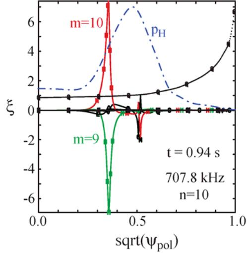
Fig. 5. NOVA calculated eigenfunction for the  $n=10$  upper gap mode at 707.8 kHz for  $t=0.94$  s in H-mode showing the dominant poloidal harmonics  $m=9, 10$ . The  $q$  profile and normalized fast ion pressure profile,  $p_H$ , are also shown.
