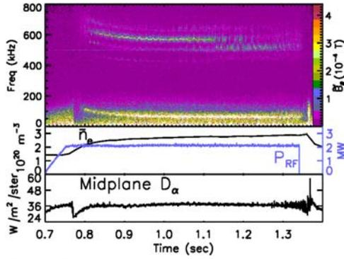
Fig. 2. Fourier spectrogram of a poloidal field pick-up coil signal during an EDA H-mode showing a QCM and several high frequency TAEs. The line averaged density, ICRF power, and  $D_\alpha$  emission are also shown.
