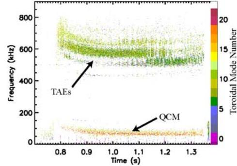
Fig. 3. Toroidal mode number color spectrum vs. time for the discharge shown in Fig. 1. The QCM and TAEs all rotate in the electron direction. The TAEs have  $n$  numbers between 6 and 11.
