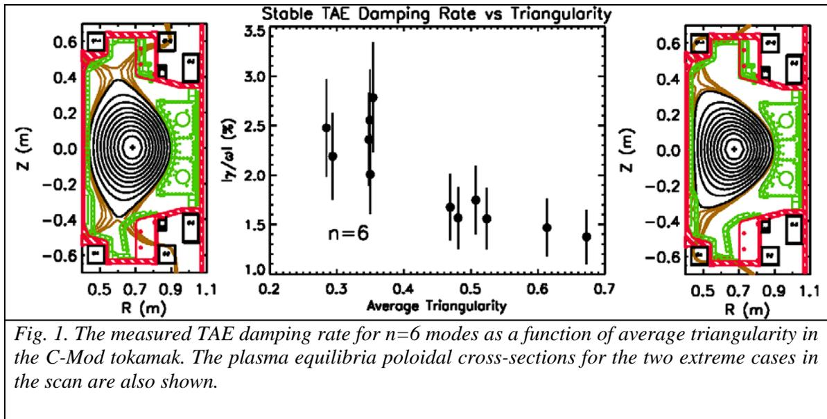
Fig. 1. The measured TAE damping rate for  $n=6$  modes as a function of average triangularity in the C-Mod tokamak. The plasma equilibria poloidal cross-sections for the two extreme cases in the scan are also shown.
