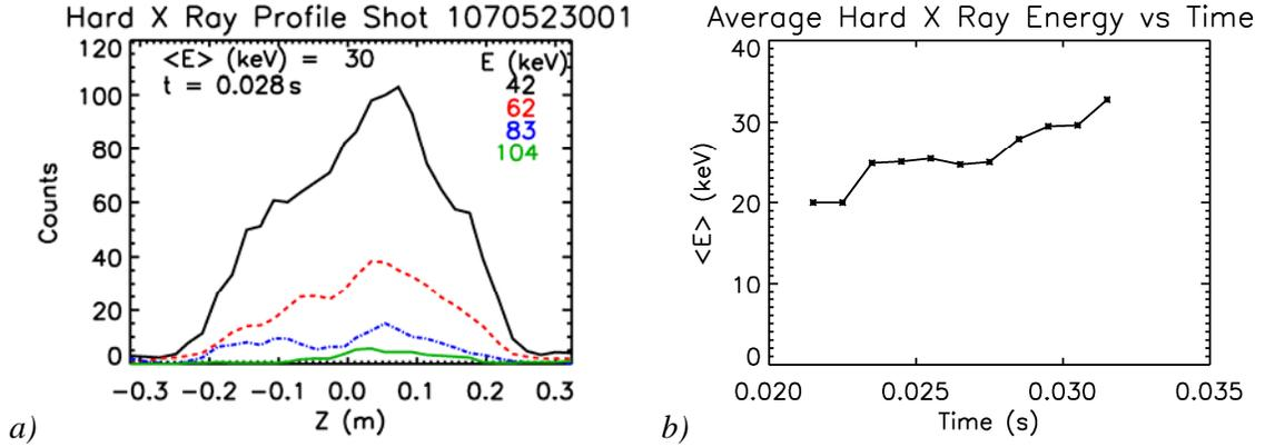
Fig. 8. a) Measured hard x ray line integrated profile for energy bins from 42 to 104 keV at the time of the bursting high frequency modes in Fig. 6. b) Average hard x ray energy across the profile as a function of time during the bursting high frequency modes of Fig. 6.
