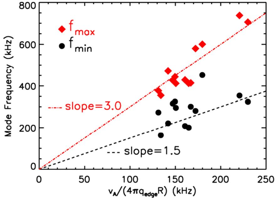
Fig. 7. Plot of the minimum and maximum mode frequencies at a given time during a series of discharges with toroidal fields ranging from 4.5 T to 6.3 T as a function of the TAE frequency, using the line averaged density in the Alfvén velocity and the edge  $q$  value. The linear dependence of the minimum and maximum frequencies indicates they are Alfvén eigenmodes.
