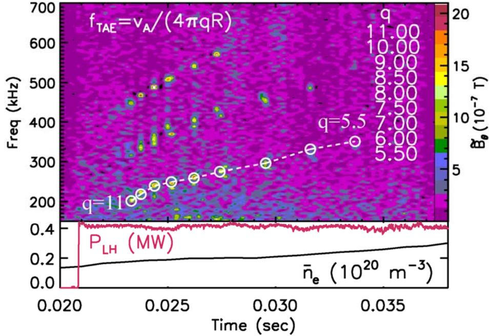
Fig. 6. Bursting high frequency modes early in the current rise with LHCD together with a fit to the center of the gap TAE frequency overlaid on each burst. The fitted resonant  $q$  values fall on integer and half integer values from 11 down to 5.5.
