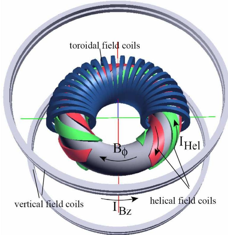
*Fig. 1 Coil system of WEGA stellarator*
