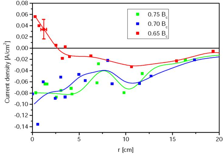
Fig. 4 Experimental current density profiles measured by a movable Rogowski coil for 6 kW injected power.
