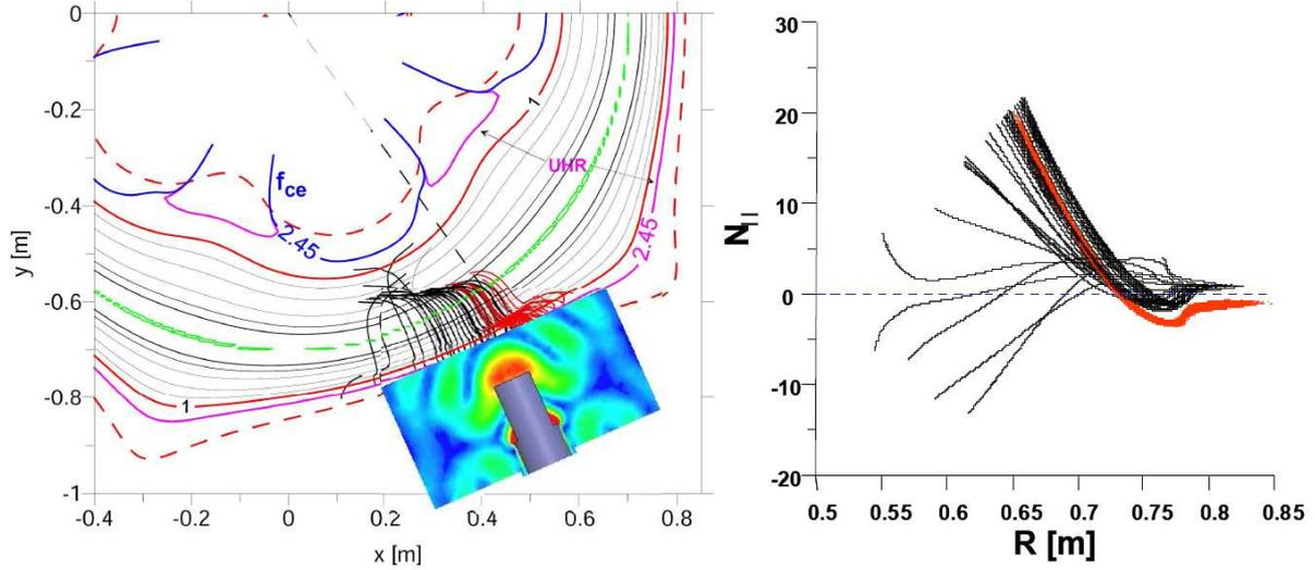
Fig. 2 left) Ray trajectories of EBW's in equatorial projection. right) Development of  $N_{||}$  during propagation until absorption for the individual EBW rays calculated by the 3D ray-tracing code.
