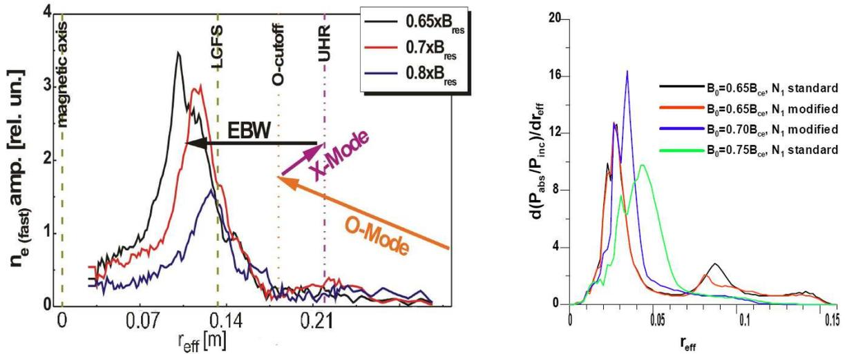
Fig. 3 Power deposition profiles for different magnetic field strength, achieved from probe measurement (left) and ray-tracing calculation (right). In addition in the sensitivity on different profiles of the supra-thermal electrons with a temperature of 150 eV was tested.
