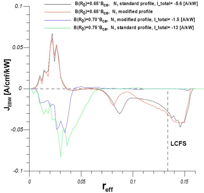
Fig. 5 Calculated current density for different central toroidal field.
