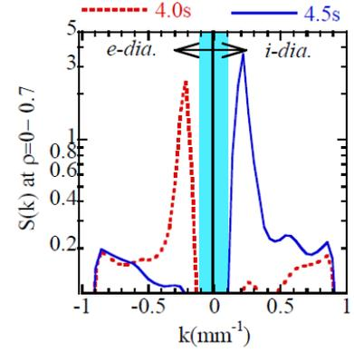
Fig.9 Wavenumber spectrum at  $\rho=0-0.7$ . Colored region  $-1<k<1mm^{-1}$  is instrumental cut off region
