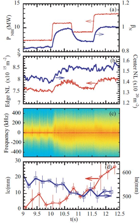
Fig.3 Time history of (a) NB power, normalized beta ( $\beta_n$ ), (b) line integrated density (c)reflected power spectrum and (d)density scale length, radial correlation length in JT-60U.
