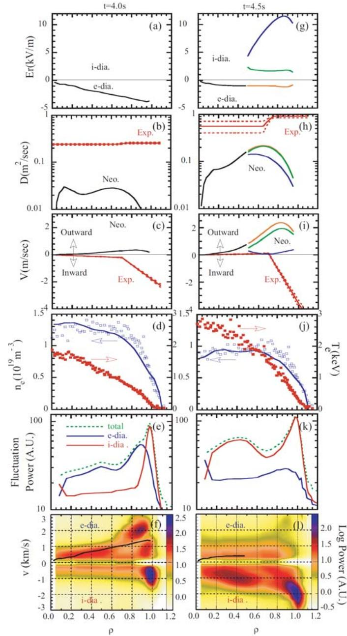
Fig.8(a), (g) Radial profile of  $E_r$ , (b), (h)  $D$ , (c),(i)  $V$ , (d),(j)  $n_e$   $T_e$ , (e), (k) fluctuation power and (f), (l) fluctuation phase velocity. (a)-(f) are at low NB power (1.1MW at  $t=4.0s$ ) and (g)-(l) are at high NB power (5.6MW at  $t=4.5s$ ). Neoclassical  $E_r \times B_t$  roation velocities are indicated by black lines in Fig.8 (f) and (l).
