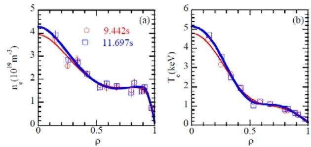
Fig.4 (a)  $n_e$  and (b)  $T_e$  profile at high (7.4MW,  $t=9.442\text{s}$ ) and low (12.8MW,  $t=11.697\text{s}$ ) NB power
