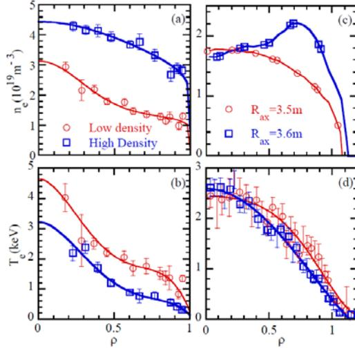
Fig. 1 (a), (c)  $n_e$ , and (b),(d)  $T_e$  profiles. (a) and (b) from JT-60U, and (c) and (d) from LHD. Here, plasmas in low and high density plasmas in JT-60U, and those at  $R_{ax}=3.5\text{m}$  and  $R_{ax}=3.6\text{m}$  in LHD are compared.
