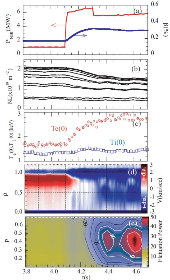
Fig.7 Time history of (a) NB heating power, diamagnetic  $\beta$ , (b) line integrated density. Higher values (upper trace) corresponds to the chord close to magnetic axis. (c) central electron and ion temperature, (d) fluctuation phase velocity and (e) fluctuation power at  $\rho=0-0.7$ .  $R_{ax}=3.6\text{m}$ ,  $B_t=2.75\text{T}$ . In Fig.7(d), red and blue colors indicate electron and ion diamagnetic direction in laboratory frame respectively.
