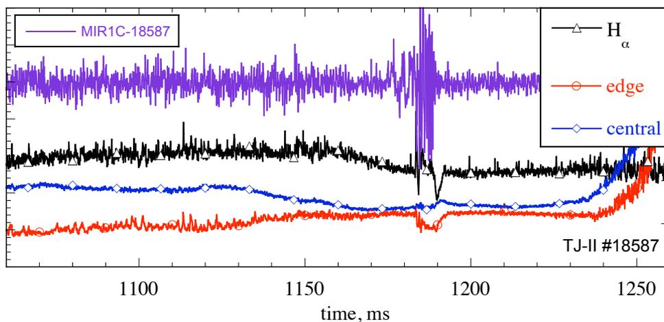
FIG. 7. From top to bottom: time traces (arbitrary units) of Mirnov coil,  $H_\alpha$  monitor, and edge and central bolometer chords for TJ-II discharge #18587.
