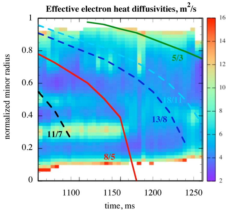
FIG. 6. Contour map of the effective electron thermal diffusivity ( $\sim 1/L_{Te}$ ) during a fast configuration change experiment. Lowest order magnetic resonances of the calculated vacuum rotational transform are traced with lines. White areas correspond to out of range data.
