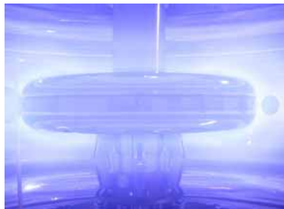
FIG.1. Magnetospheric plasma produced on the RT-1 device (viewed from a side window). A superconducting magnet is levitated in a vacuum chamber, which generates dipole magnetic field. Plasma is produced by ECH.
