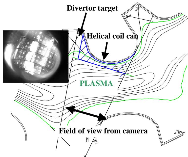
*FIG.1 A schematic drawing of the LHD horizontal plane with field of view from infrared camera and a sample image of infrared camera from this field of view. The distance from the infrared camera to the inner wall is about 5m and dust location is estimated in hatched area near the inner wall.*
