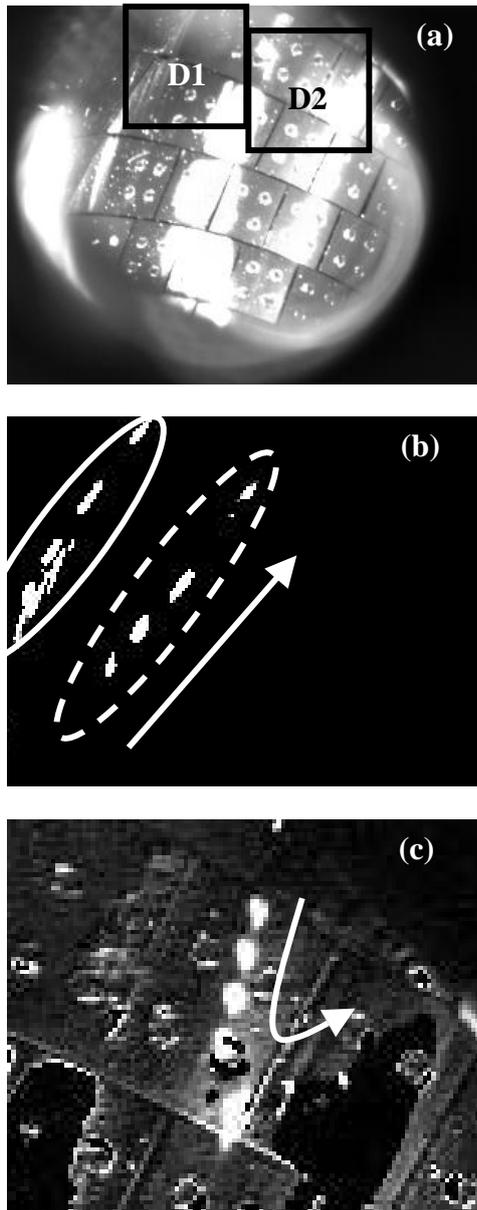
FIG.2 Movement of heated dust particles in after-glow of hydrogen plasma observed by infrared camera. (a) observed image by infrared camera. Observed areas for each dust, D1 and D2, are shown as squares (b) dust, D1, images located in ellipse by solid line and reflected images are shown by dotted line (c) dust, D2, images. Allows show moving directions.
