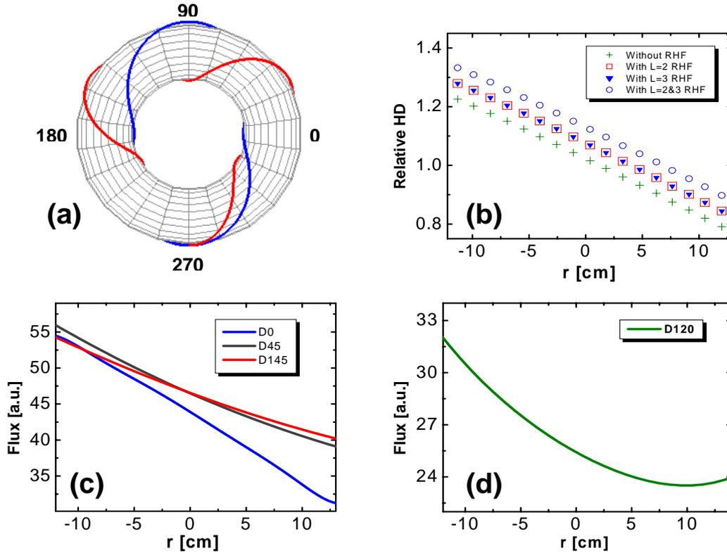
FIG. 3. a) A typical Schematic of  $L=2/1$  and  $L=3/1$  RHF winding coil around the chamber, b) Effect of RHF with different mode on plasma horizontal displacement, c) Magnetic field calculation from RHF via Bio-Sawart law in best position  $0^\circ$ ,  $45^\circ$ ,  $145^\circ$  for installing Sine-Coil, d) A sample magnetic field calculated in the  $120^\circ$  as a high nonlinear effective position.
