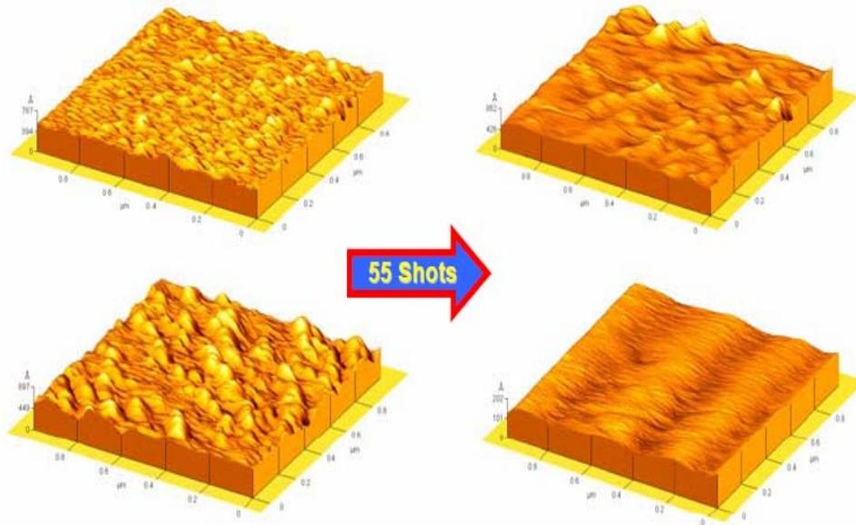
FIG. 4. Changes in roughness at two different positions of the sample with respect to plasma core. Below one is closer to plasma core. Left figures are before discharges and right figures are after discharge.
