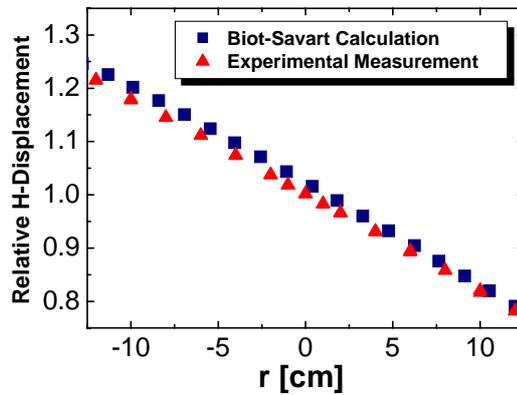
FIG. 1. Comparison of calculations with actual plasma position. The rectangle and the triangle symbols show the Biot-Savart law calculation and the measurements with the sine-coil, respectively.
