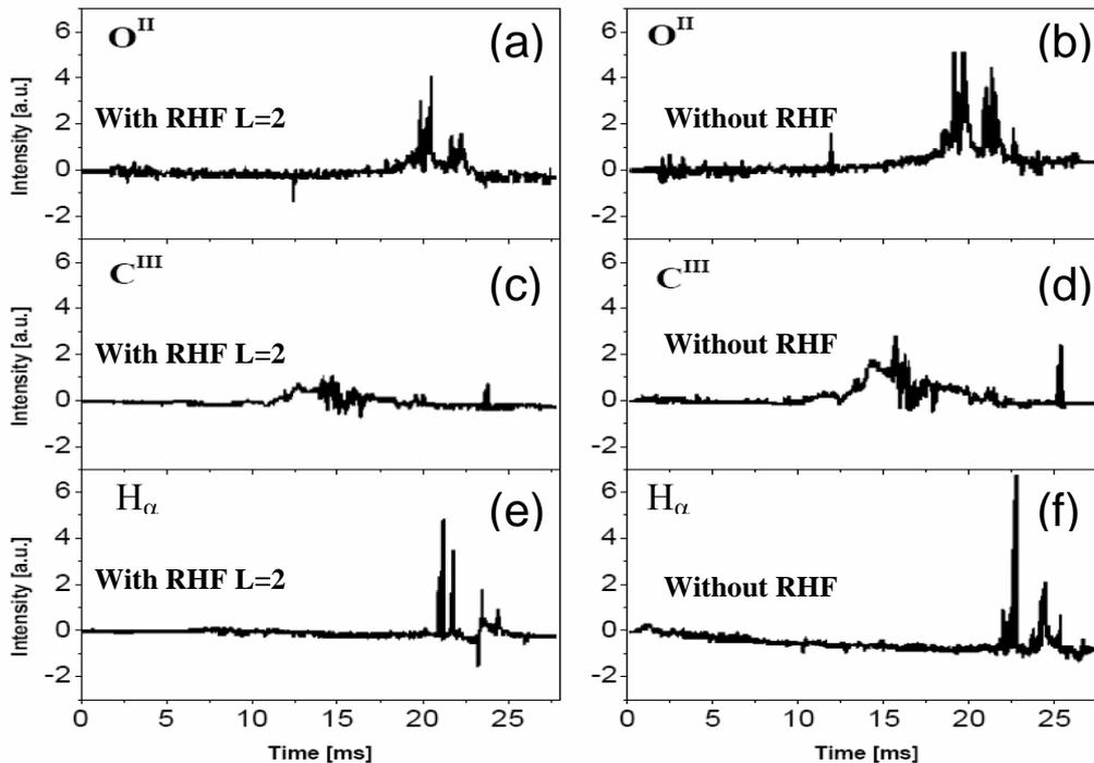
FIG. 2. The measurement results of visible line emissions of  $O^{II}$  (a, b),  $C^{III}$  (c, d) impurities and  $H_{\alpha}$  radiation (e, f) with and without RHF ( $L=2$ ).
