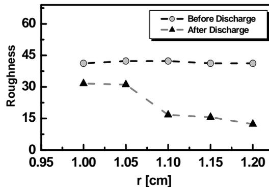
FIG.5. Profile of comparing roughness of samples before discharge and after discharges, where,  $r$  (normalized) is the position of samples with respect to plasma core.
