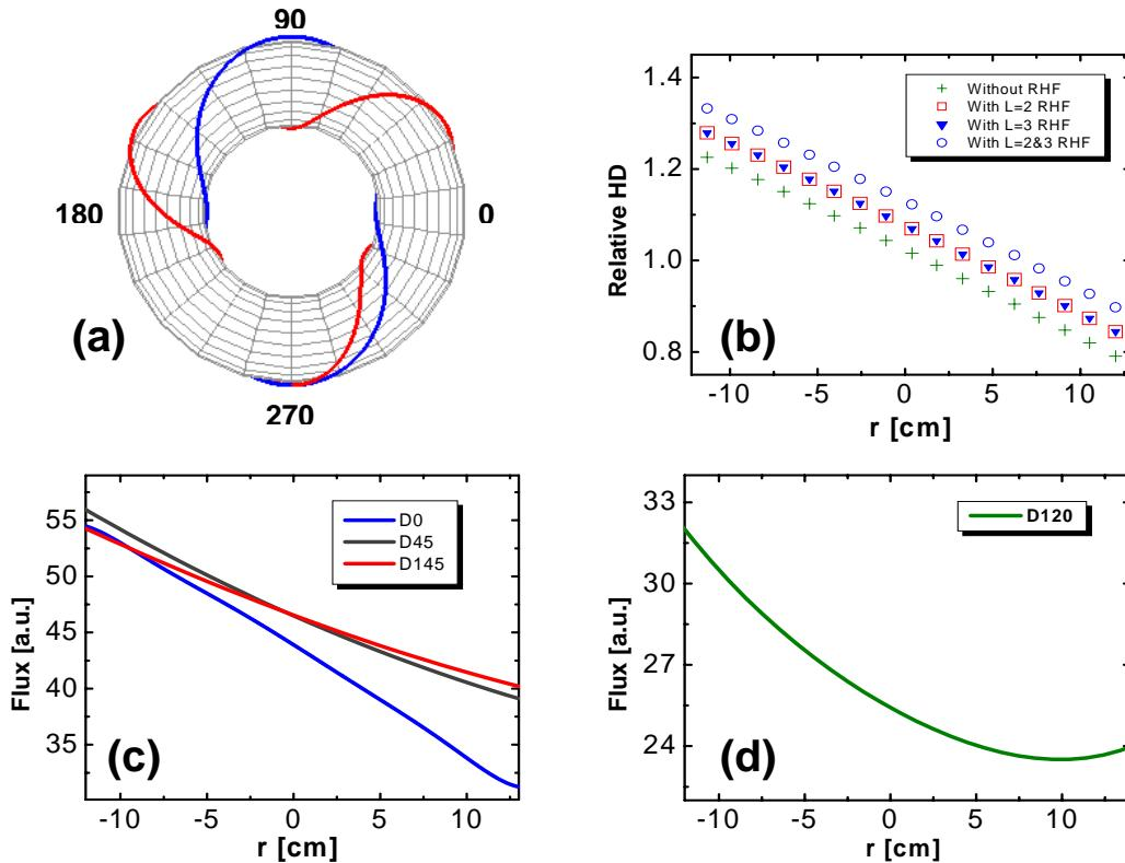
*FIG. 3. a) A typical Schematic of L=2/1 and L=3/1 RHF winding coil around the chamber, b) Effect of RHF with different mode on plasma horizontal displacement, c) Magnetic field calculation from RHF via Bio-Sawart law in best position 0°, 45°, 145° for installing Sine-Coil, d) A sample magnetic field calculated in the 120° as a high nonlinear effective position.*
