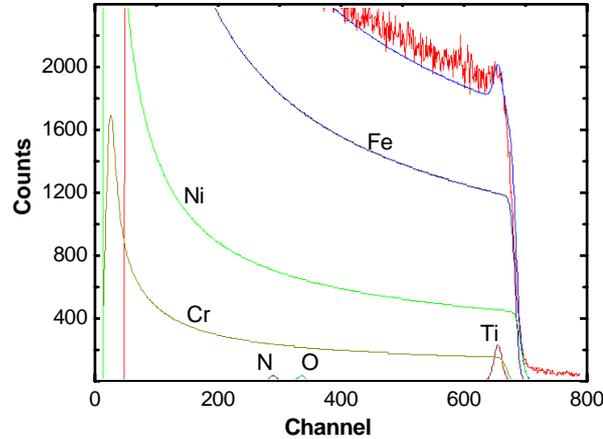
FIG. 6. The analyses of RBS measurements with SIMNRA Code.
