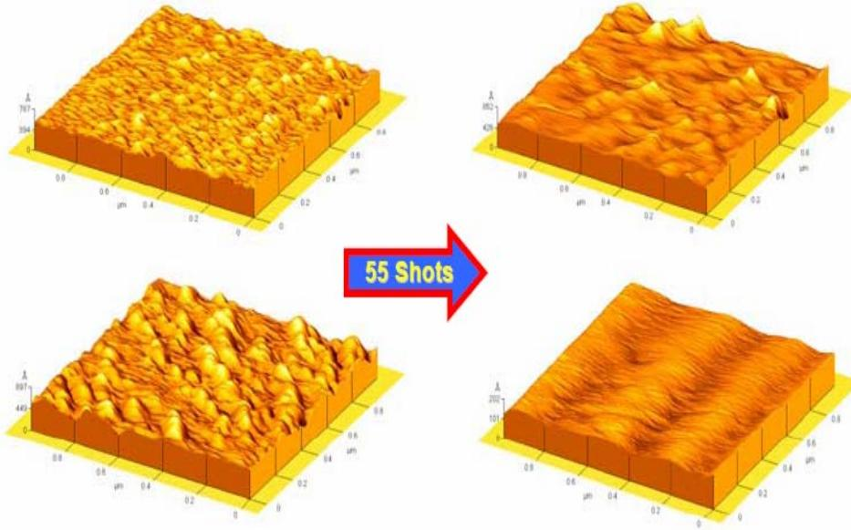
*FIG. 4. Changes in roughness at two different positions of the sample with respect to plasma core. Below one is closer to plasma core. Left figures are before discharges and right figures are after discharge.*
