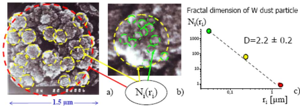
Fig.8. QSPA dust hierarchical structure (a,b) and fractal dimension (c).
