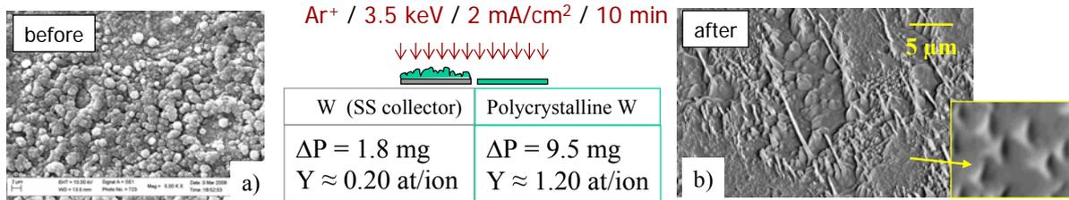
Fig.5. Ar<sup>+</sup> sputtering of W dusty film. a) before modification (b) after modification
