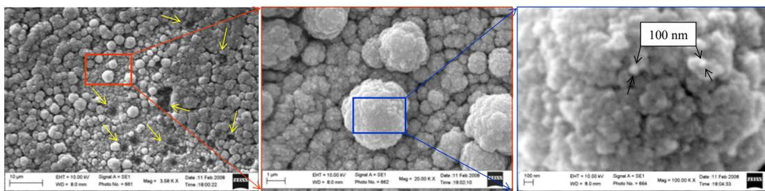
Fig.2. QSPA. Dust particles after W target erosion with 1.5 MJ/m<sup>2</sup> energy load.
