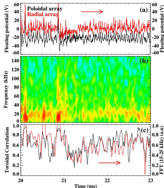
**Figure 4:** Time evolution of: (a)  $V_f$  measured simultaneously in two toroidal positions at  $r-a = -10$  mm; (b)  $V_f$  spectrogram; and (c) toroidal correlation between  $V_f$  signals together with the amplitude of the  $V_f$  power spectrum in the range 15-25 kHz.
