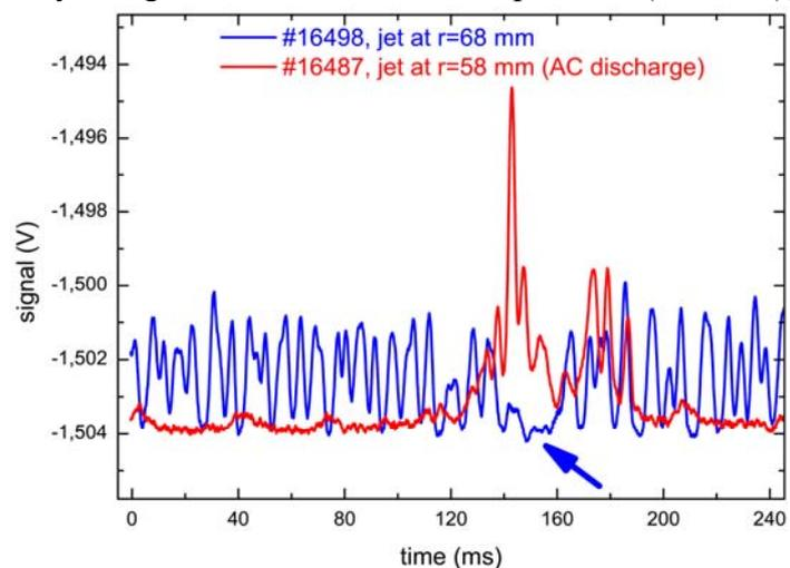
**Figure 1:** Signal response of the IR sensor for two different radial positions of the of the gallium injector.
