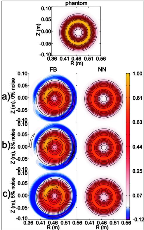
**Figure 2:** Comparison of the reconstructions using Fourier-Bessel and Neural Networks algorithms for different ranges of measurement noise - a) has no noise, b) has 3% noise and c) has 5% noise. Clearly, the NN reconstructions are superior to the FB in any of the cases presented.
