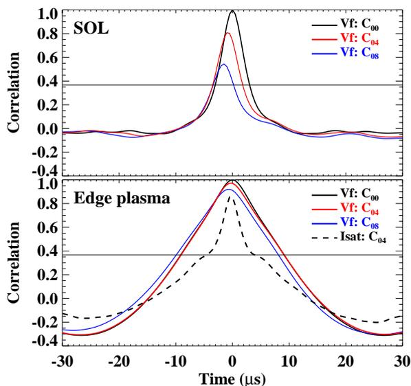
**Figure 3:** Floating potential cross-correlation for pins poloidally separated by 4 ( $C_{04}$ ) and 8 mm ( $C_{08}$ ) measured in the SOL and in the edge plasma. The  $V_f$  auto-correlation is also shown ( $C_{00}$ ) as well as the  $I_{sat}$  cross-correlation in the edge plasma.
