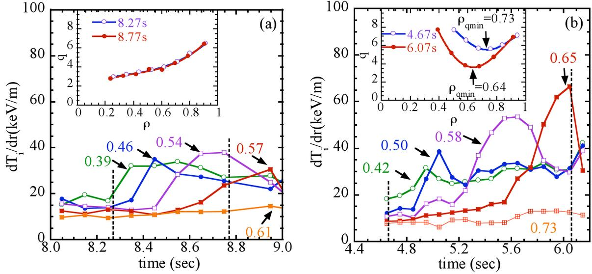
FIG.2 Time evolution of temperature gradients at various normalized radii (evaluated at  $t = 8.3s$  in Fig(a) and  $5.0s$  in Fig(b) and indicated in the figures with numbers) during the formation of the ITB with (a) the positive magnetic shear and (b) the negative magnetic shear in JT-60U.
