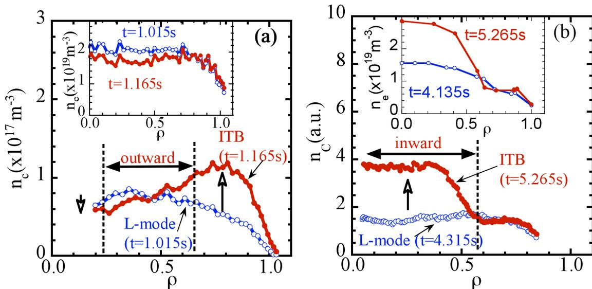
FIG.4 Radial profiles of electron density and carbon density ( $n_C$ ) in the L-mode phase and ITB phase in (a) LHD and (b) JT-60U plasmas. Associated with the formation of an ITB, a strong outward convection leads the  $n_C$  profile to be hollow in the LHD plasma, while a strong inward convection is observed in the ITB region of the JT-60U plasma.
