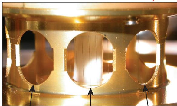
Outer array    Foam target    Inner array
