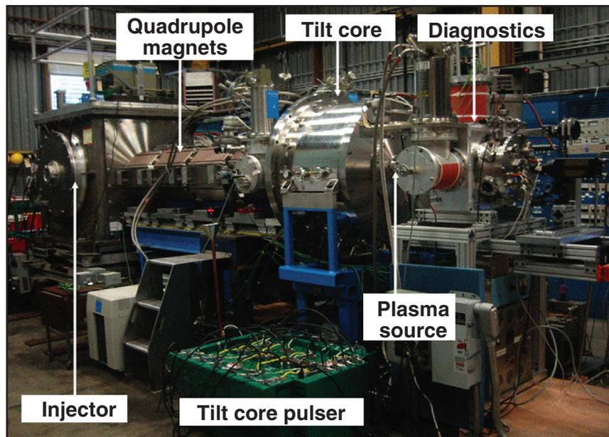
A 200-ns, 300-keV  $K^+$  ion beam is compressed to a few nanoseconds
