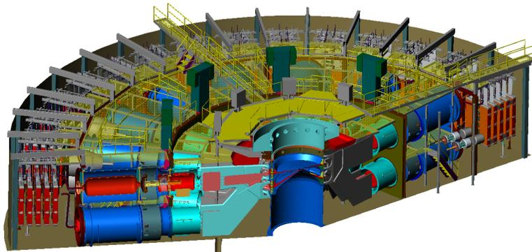
The ZR project is upgrading the performance of Sandia's "Z"-pinch facility
