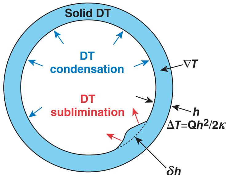
The temperature gradient can also be established by heating externally (IR radiation).<sup>2</sup>
