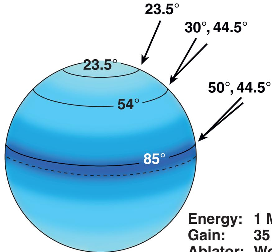
The required intensity variations on target can be achieved through a combination of spot shape, pulse shape, and beam pointing.
