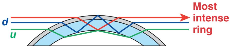
Refracted light creates a bright ring in a backlit image
