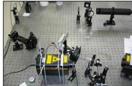
Mirror-steering test using target glint
