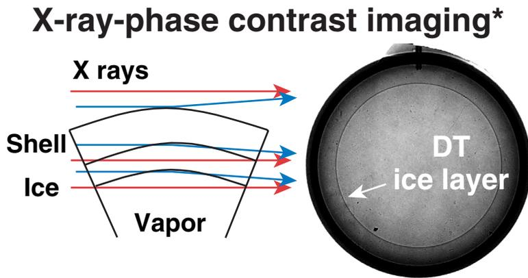
Higher-mode roughness is apparent at 18.3 K
