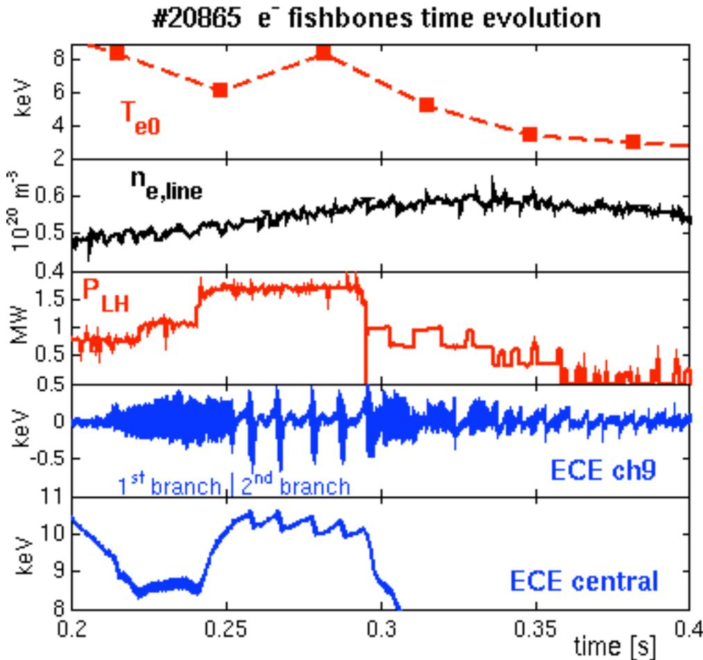
*FTU  $e^-$  fishbones*: LH power alone in low  $n_e$  and  $\sim$ full CD
