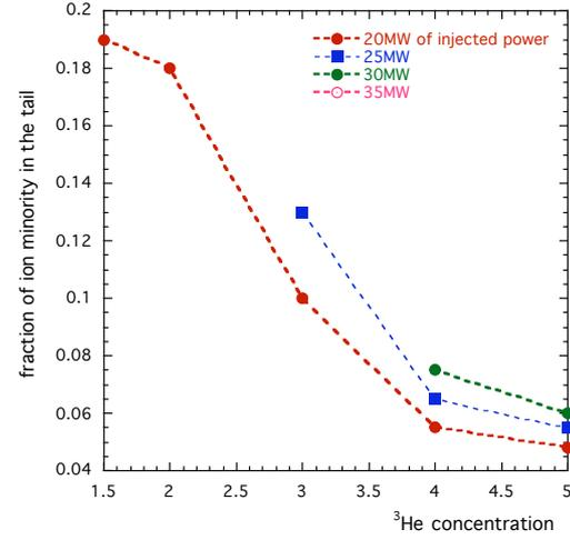
FIG.8. Minority fraction of the tail at the peak vs the minority concentration.
