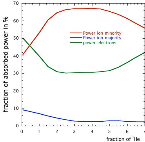
FIG.1. Fraction of absorbed power vs the minority concentration at fixed  $n_{\parallel}=5$ , for the plasma parameters of the H-mode scenario.
