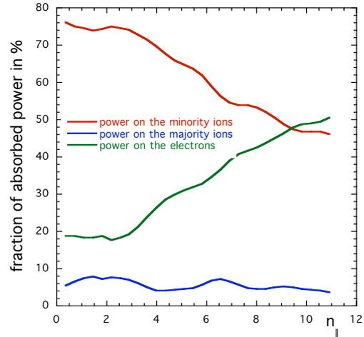
FIG.2. Fraction of absorbed power vs the parallel wave-number at fixed  $^3\text{He}$  concentration 2%, for the plasma parameters of the H-mode scenario.
