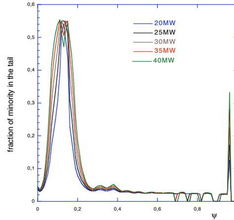
FIG.10. Minority fraction of the tail vs the flux coordinate and for plasma parameters  $n_0 = 1.93 \times 10^{20} m^{-3}$  and  $T_0 = 14.5 KeV$ .
