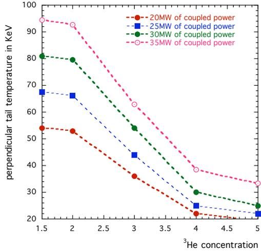
FIG.7. Perpendicular temperature of the tail at the peak vs the minority concentration.
