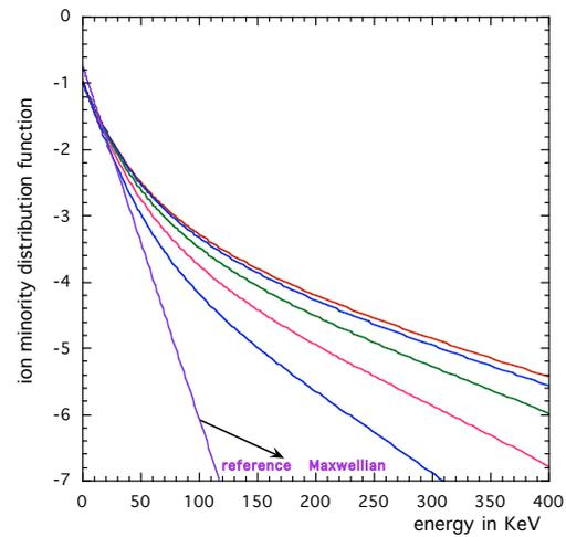
FIG.4. Ion minority distribution function vs the energy for several values of the pitch angle.
