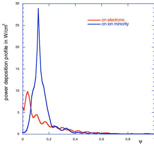
FIG.3. Power deposition profiles vs the plasma radius and for the various species.
