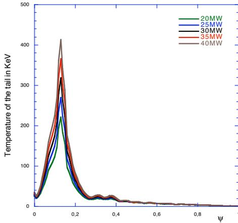
FIG.9. Perpendicular temperature of the tail vs the flux coordinate and for plasma parameters  $n_0 = 1.93 \times 10^{20} m^{-3}$  and  $T_0 = 14.5 KeV$ .
