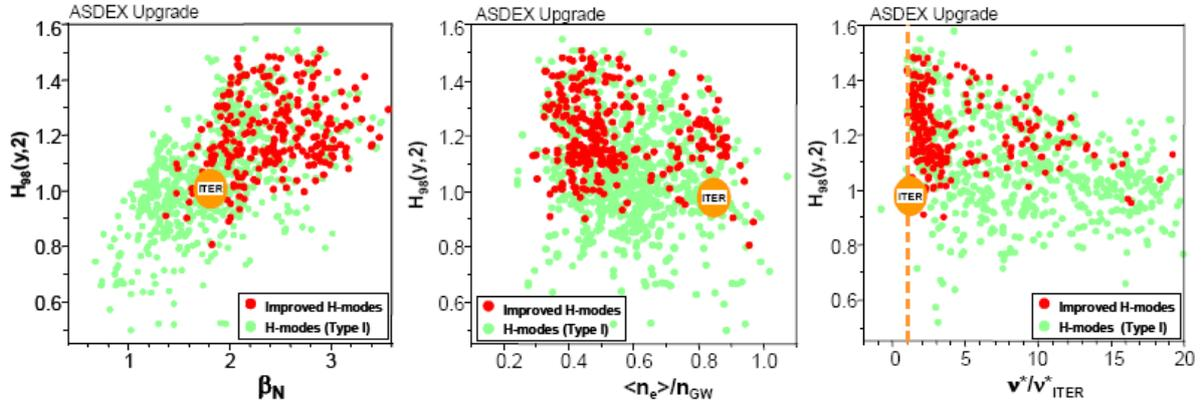
Fig. 11: Confinement factor  $H_{98}(y,2)$ , of improved and ELMy H-modes in terms of  $\beta_N$ , line averaged density norm. to Greenwald density ( $\langle n_e \rangle / n_{GW}$ ), and collisionality norm. to the ITER collisionality ( $v^* / v_{ITER}^*$ )
