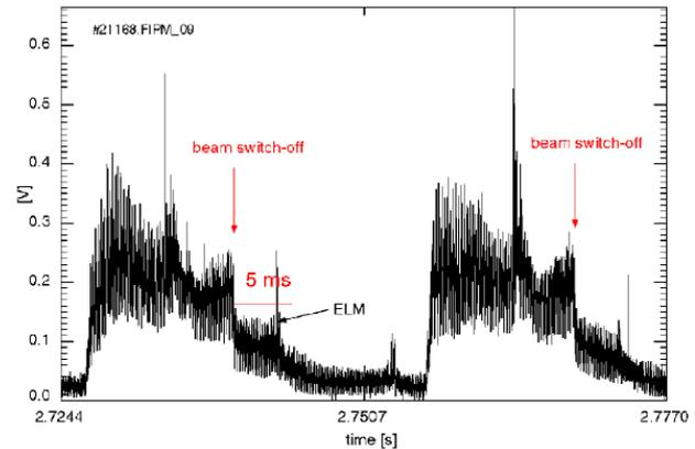
Fig. 4: Response of the fast ion losses to switch-on and -off of the NBI source for particles deposited on the low field side
