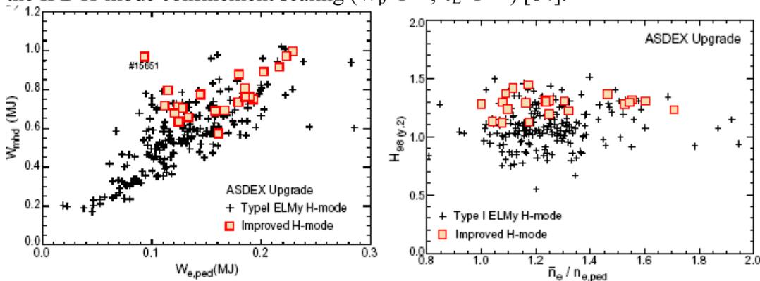
Figure 10: Edge-core relation in improved H-mode and type I ELMy H-mode data sets: (a) total MHD stored energy vs. pedestal electron energy. (b)  $H_{98(y,2)}$  vs. density peaking factor,  $n_e/n_c(\rho=0.9)$ .
