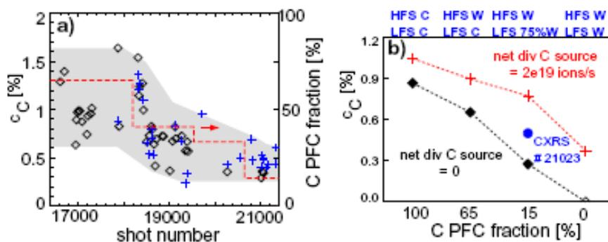
Figure 6: a) Long term development of the carbon concentration in the outer core plasma during a high density standard H-mode phase as measured by CXRS with NBI injector 1 (diamonds) and 2 (crosses). The dashed lines indicate the fraction of PFC carbon coverage. b) Modelling of the C concentration with changing W coating in AUG with and without net C ion influx from the divertor.
