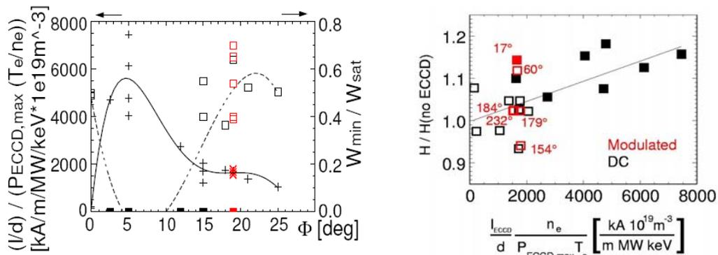
Fig. 4 : Normalized ECCD current density  $I_{\text{ECCD}}/d$  (from TORBEAM calculations) as function of the toroidal launching angle  $\Phi$  (black crosses) together with the experimentally achieved normalised minimal island size  $W_{\text{min}}/W_{\text{sat}}$  of (3/2)-NTM.
