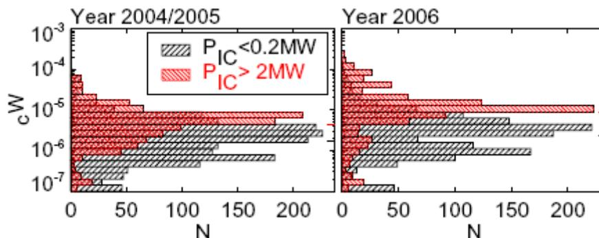
Figure 7: Distributions of tungsten edge concentration with (red) and without (black) considerable ICRF heating for the campaign 2006 with tungsten limiters in comparison to two previous campaigns with graphite limiters. Bars at the right hand side give mean values[67].
