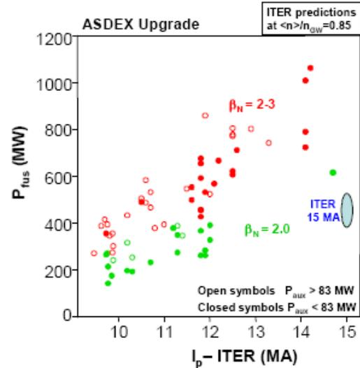
Fig. 13: Prediction of the fusion power in ITER from scaling up kinetic profiles data from ASDEX Upgrade. Input power requirements ( $P_{aux}$ ) to sustain the  $\beta_N$  in ITER as obtained in ASDEX Upgrade for the IPB confinement scaling law.
