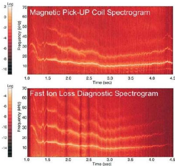
Fig.3 : NTM (magnetic signals, ~5-20 kHz and harmonics) induces fast particle losses measured by fast ion loss detector.
