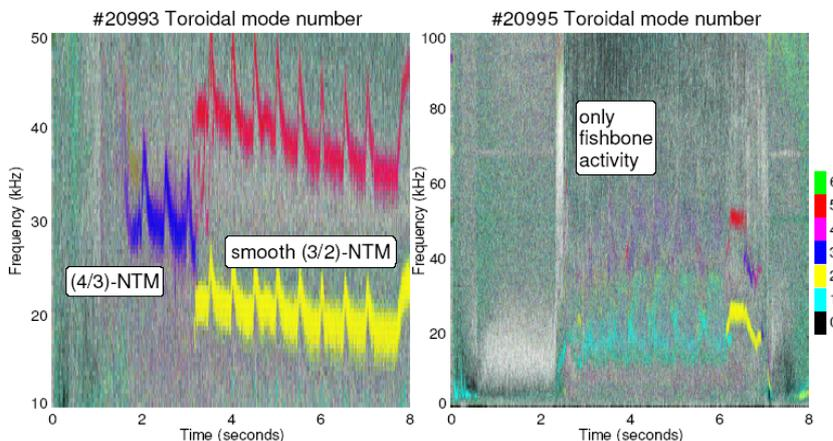
Fig. 9: MHD activity of early-heating (left) and late-heating (right) improved H-mode scenarios in divertor configuration.
