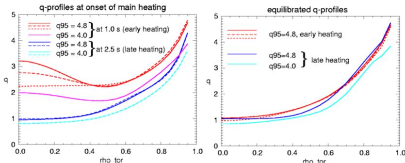
Fig. 8: Variation of  $q$ -profiles at the onset of the main heating (left) and equilibrated current profiles (right) obtained by modification of the ramp-up phase. Red: early heating  $q_{95}=4.8$ , magenta: early heating  $q_{95}=4.0$ , blue: late heating  $q_{95}=4.8$ , cyan: late heating  $q_{95}=4.0$ . For the latter two, dashed lines refer to reproductions.
