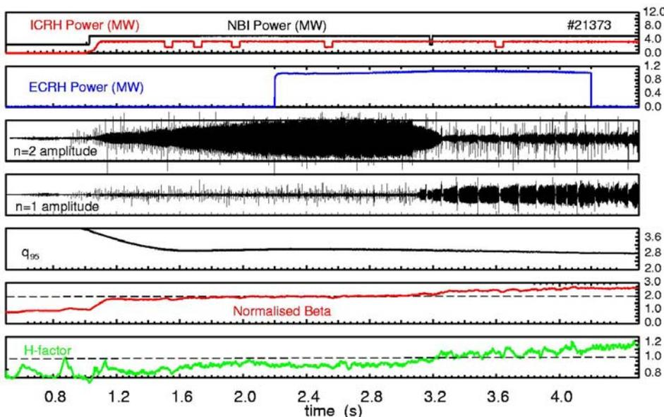
FIG. 12. Stabilisation experiment of a (3,2) NTM by sweeping ECCD over the  $q=1.5$  surface using a mild  $B_t$  ramp with a narrow deposition profile ( $W/(2d)=0.6$ ) in an improved H-mode at  $q_{95} = 2.9$ .
