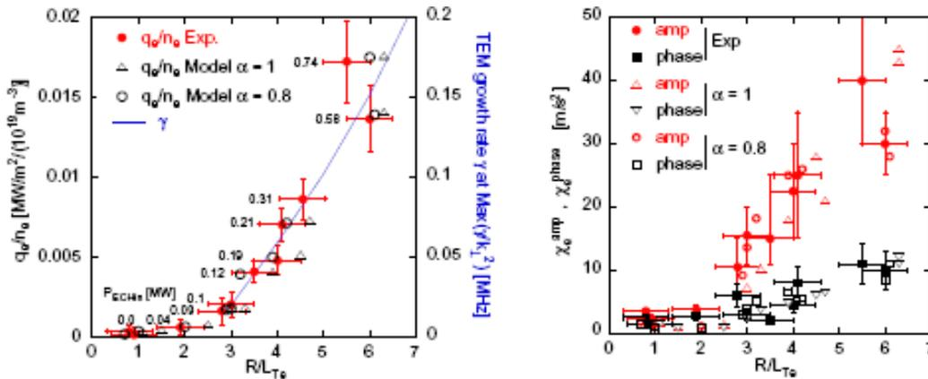
Figure 1. TEM threshold. Left: electron heat flux versus  $R/L_{Te}$ , experimental data, simulations with empirical model and growth rate of the TEM.
