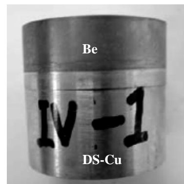
Fig. 1. The Be/Cu joint by HIP.
