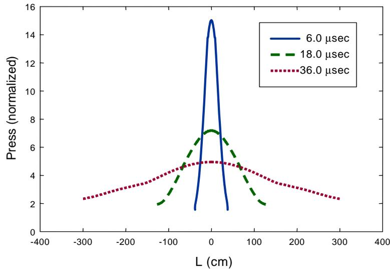
FIG. 6. Pellet cloud pressure along magnetic field line normalized to the background plasma pressure at the start location of the cloudlet drift. The profile is shown for different times after the cloudlet is detached from the pellet and starting to drift. 0 on the X axis is the pellet location.
