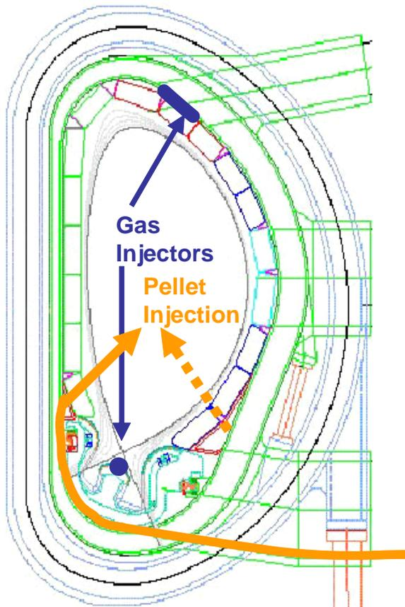
FIG. 1. Cross section of ITER showing the pellet injection and gas injection locations. The dashed pellet trajectory is the proposed low field side location for ELM triggering.
