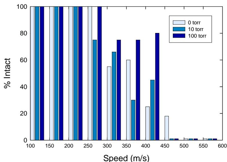
FIG. 2. Guide tube test results showing percent of intact pellets at different speeds for the inner wall guide tube mockup. Tests were performed at 3 different pressures in the guide tube.
