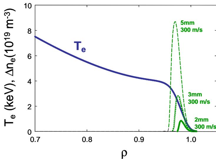
FIG. 5. Electron temperature profile in the outer 1/3 of the ITER plasma overlaid with calculated pellet mass perturbations from different size and speed pellets injected from the proposed outer wall injection line.
