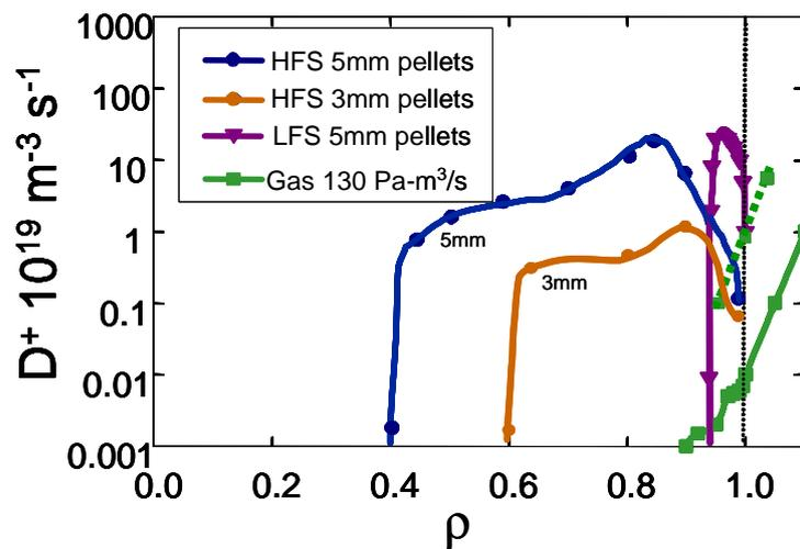
FIG. 4. Comparison of pellet fueling and gas fueling source profiles for ITER using the specified 16 Hz 5-mm pellets and  $130 \text{ Pa}\cdot\text{m}^3/\text{s}$  ( $1000 \text{ torr}\cdot\text{L}/\text{s}$ ) of gas. The dashed gas curve is calculated from the SOLPS code in actual ITER geometry. The solid gas curve is from a B2-Eirene slab calculation.
