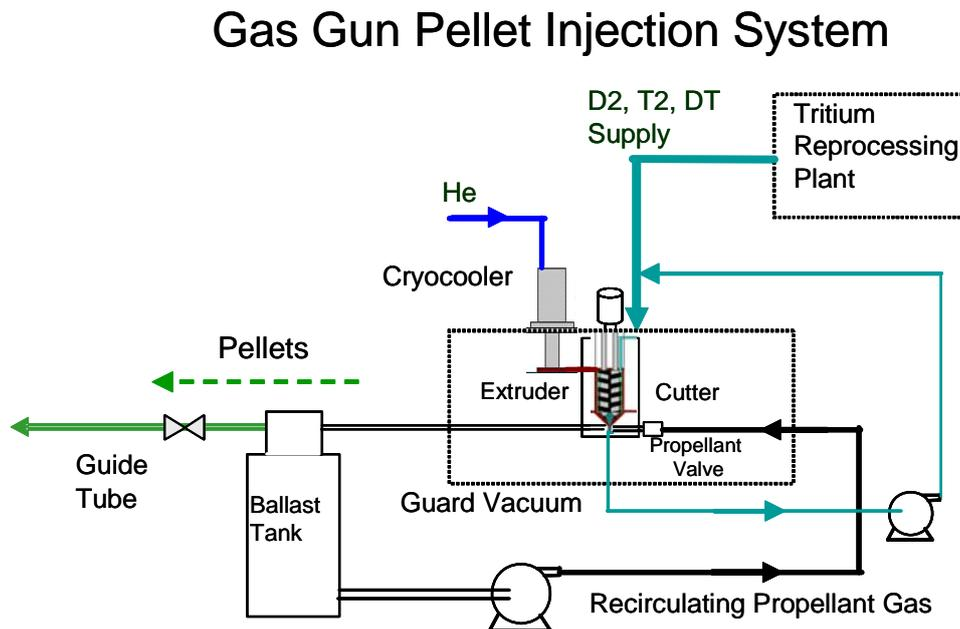
FIG. 3. Block diagram of the proposed gas gun pellet injection system for ITER.
