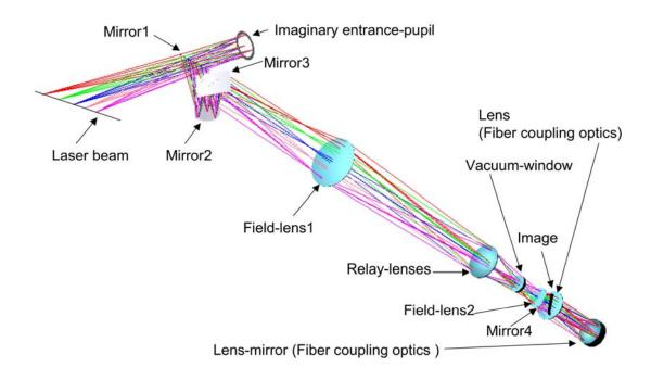
FIG. 4. Layout of in-vessel collection optics for Edge Thomson scattering.
