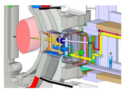
FIG. 1. Outline schematic of the port plug area LIDAR design for ITER.
