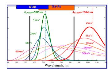
FIG. 2. Scattered spectral power density for Nd:YAG fundamental and 2nd harmonic wavelengths. Inserts show matching of different wavelengths to the spectral response of two types of photocathodes (S-20, GaAs).
