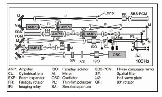
FIG.3. Laser optical design for edge Thomson scattering. High laser efficiency using Cr;Nd:YAG ceramic rods (efficiency is 2 times). Dual beam output to increase laser energy and to avoid laser damage.
